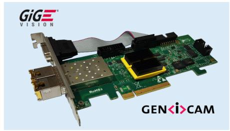
The Gidel HawkEye-20GigE frame grabbing and real-time image processing system offers true 10 GigE acquisition capabilities guaranteeing 100% frame capture with no frame loss. The board is supported by comprehensive system I/Os, ROI capture capability, multi-link aggregation and chunk data (payload type: 0x4001) transmission.
