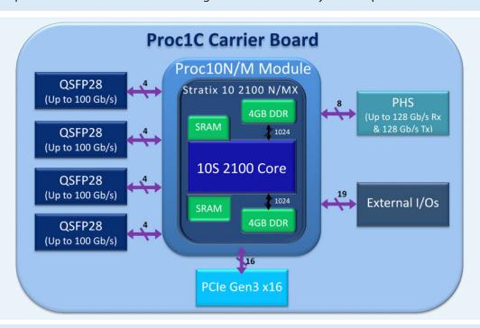
The off-the-shelf carrier-board solution supports: PCle Gen.3 x16 host interface, 4 x QSFP28 for up to 400 Gb/s aggregated bandwidth, Gidel PHS connector for mounting daughterboards, and 19 x GPlOs for peripheral system control. The PHS offers up to 128 Gb/s Rx/Tx enabling, for example, to connect 8x CoaXPress-12 cameras\*.
