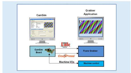
The Gidel **CamSim™** is a flexible high-performance camera simulator that generates CoaXPress and camera link video stream and test patterns for testing frame grabbers or vision/imaging systems. The system supports all CoaXPress and Camera Link™ v2.0 configurations.
