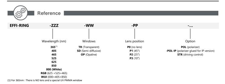
Please note that with the polarizer accessory, the EFFI-Ring is IP50. For IP65 polarized version, choose -POL-IP option.
