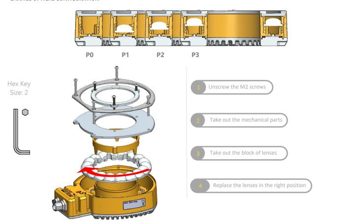
To handle the optical components, wearing gloves is strongly recommended.
