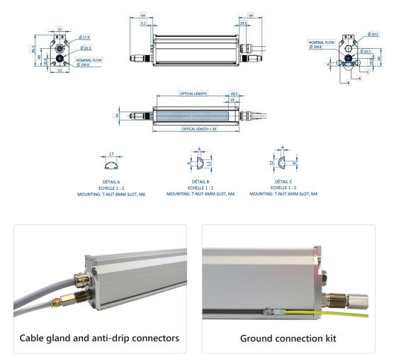
Note 1: The anti-drip connectors for watercooling only fit 8mm diameter tubes (PVC recommended).Note 2: Two tubes must be provided by the customer for watercooling (one for each side of the product).Note 3: The ground connection kit is provided in a separated bag and must be set by the customer.
