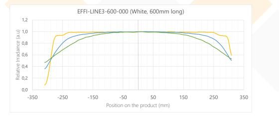
0mm working distance — 100mm working distance — 300mm working distance
