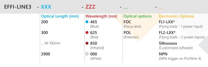
\*XX=Cable Length in meter [2/ 5 / 10] - L5 is the defaut configuration if the length is not specified
