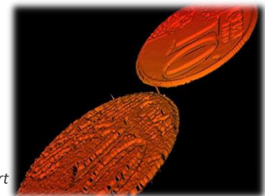
EFFI-Lase (up) vs. Laser (down): No speckle = more precision
