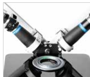
Scheimpflug telecentric optics for both projection and imaging at 90°.
