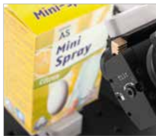
MCSM1-01X imaging a sample from an angled point of view.
