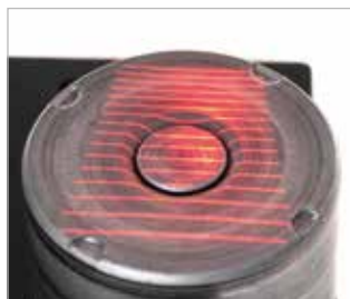
MCSM1-01X combined with a Scheimpflug projector at 90°.
