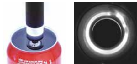
Defect and impurities detection inside containers.
