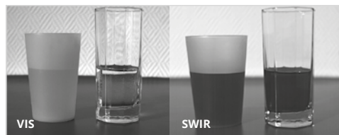
Liquid level inspection
