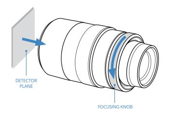
Rotate the focusing knob **clockwise** to move the lenses **away from the detector** and focus objects positioned closer to the optics.
