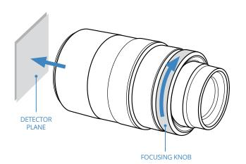
Rotate the focusing knob **counter-clockwise** to move the lenses **closer to the detector** and focus objects positioned further away from the optics .
