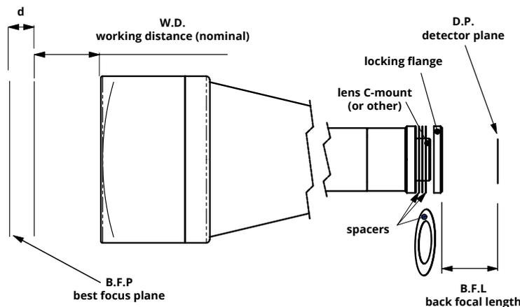
The lens back focal length is set to the C-mount standard, 17.52 mm (or other required mount) by factory default. Since many industrial cameras are not perfectly compliant, you may be required to adjust the back focal length as described behind.
