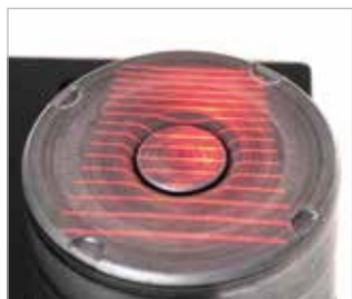
MCSM1-01X combined with a Scheimpflug projector at 90°.
