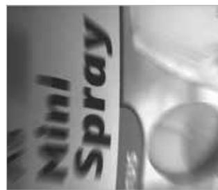
Without tilt adjustment, the object is not homogeneously focused.
