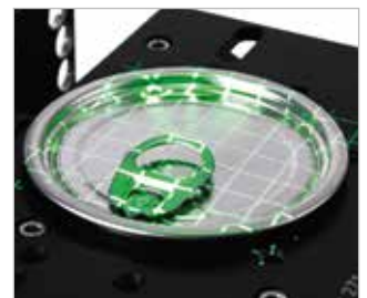
MCSM1-01X working at 45° with a pattern projector for 3D shaping.
