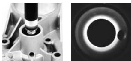
Inspection of holed parts of an engine.
