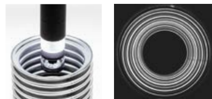
Tube scanning for integrity inspection.
