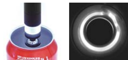
Defect and impurities detection inside containers.
