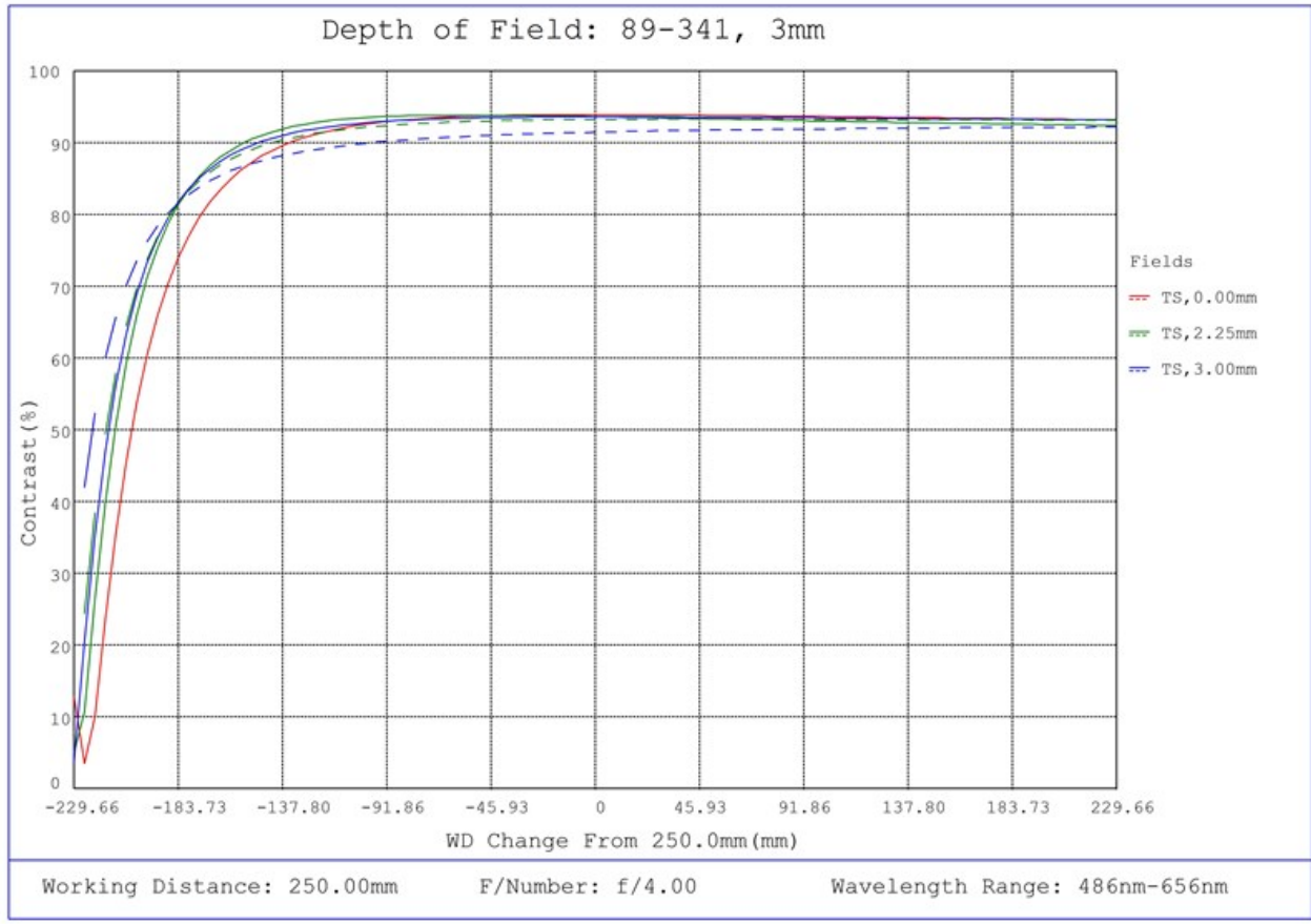
#89-341, 3mm FL f/4.0, Blue Series M12 Lens, Depth of Field Plot, 250mm Working Distance, f4
