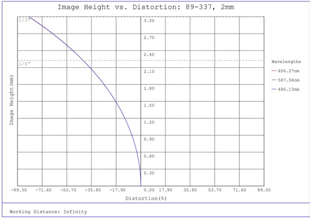
#89-337, 2mm FL f/4, Blue Series M12 Lens, Distortion Plot
