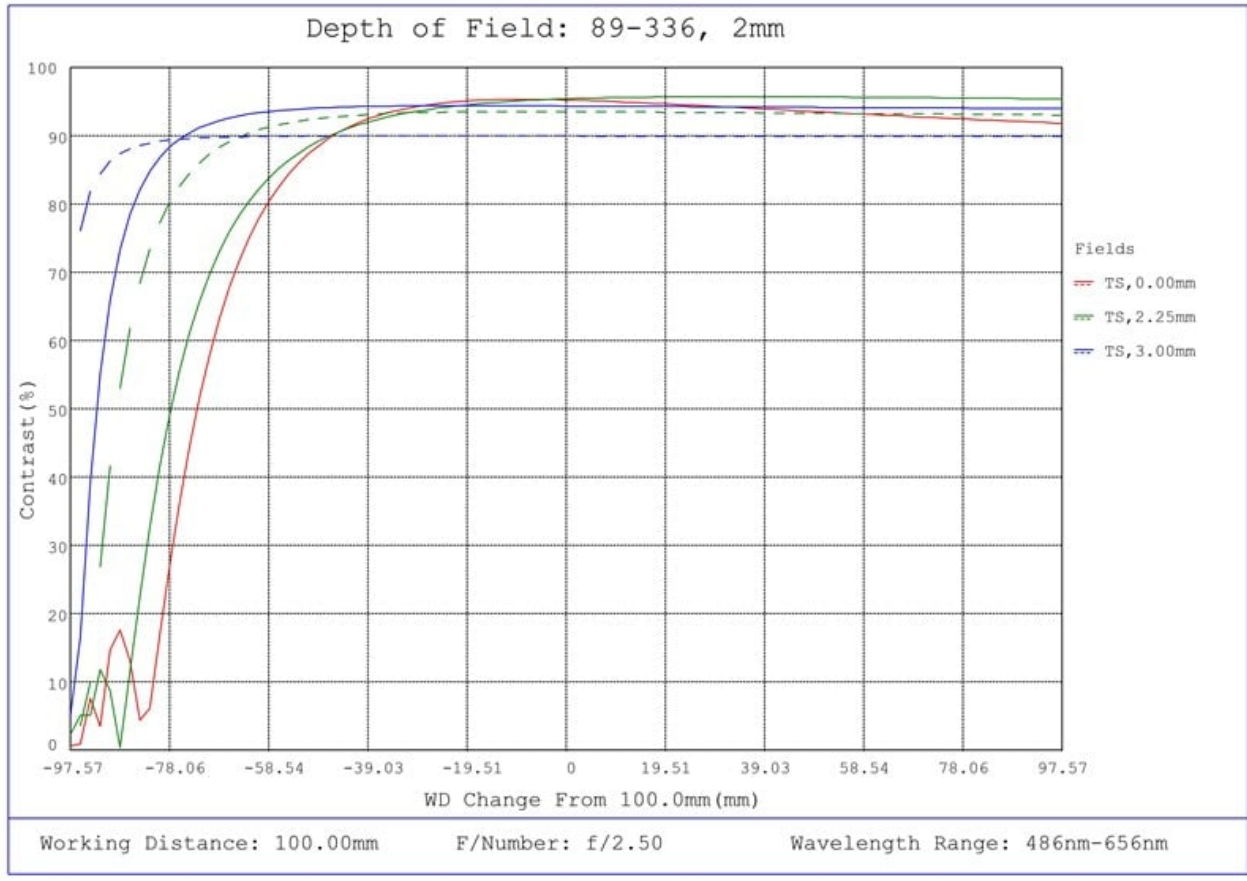
#89-336, 2mm FL f/2.5, Blue Series M12 Lens, Depth of Field Plot, 100mm Working Distance, f2.5
