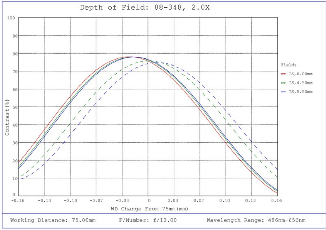
#88-348, 2.0X In-Line Illumination SilverTL™ Telecentric Lens, Depth of Field Plot, 75mm Working Distance, f10
