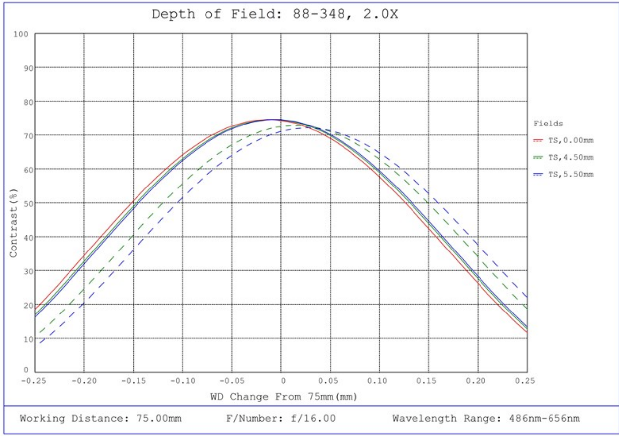
#88-348, 2.0X In-Line Illumination SilverTL™ Telecentric Lens, Depth of Field Plot, 75mm Working Distance, f16
