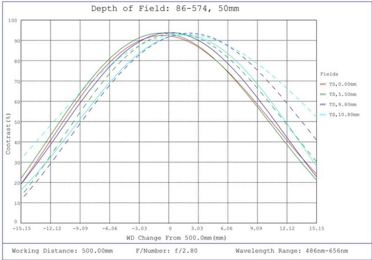
#86-574, 50mm Focal Length, HP Series Fixed Focal Length Lens, Depth of Field Plot, 500mm Working Distance, f2.8
