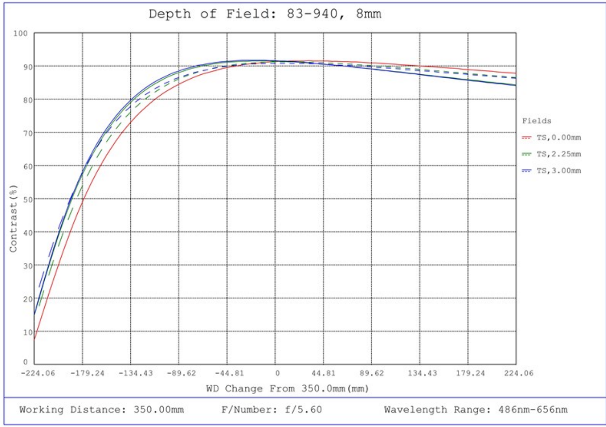
#83-940, 8mm FL f/5.6, Blue Series M12 Lens, Depth of Field Plot, 350mm Working Distance, f5.6
