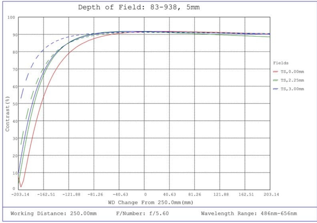
#83-938, 5mm FL f/5.6, Blue Series M12 Lens, Depth of Field Plot, 250mm Working Distance, f5.6
