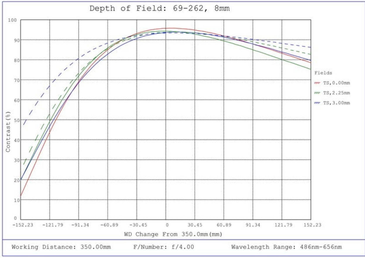
#69-262, 8mm FL f/4, Blue Series M12 Lens, Depth of Field Plot, 350mm Working Distance, f4
