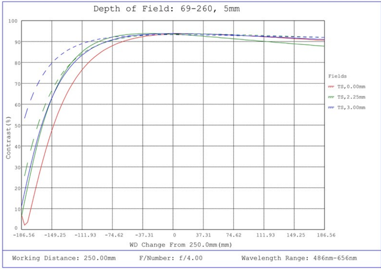
#69-260, 5mm FL f/4, Blue Series M12 Lens, Depth of Field Plot, 250mm Working Distance, f4
