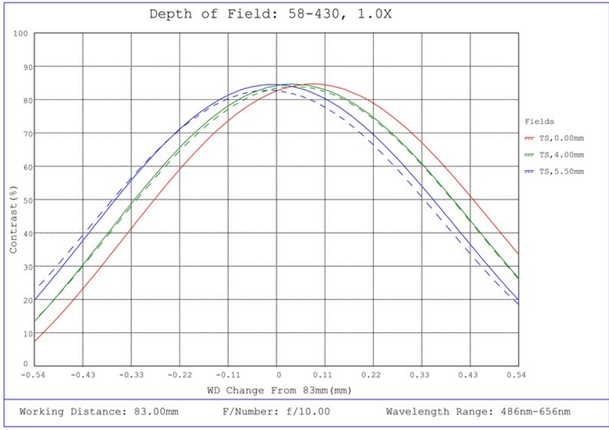
#58-430, 1.0X SilverTL™ Telecentric Lens, Depth of Field Plot, 83mm Working Distance, f10
