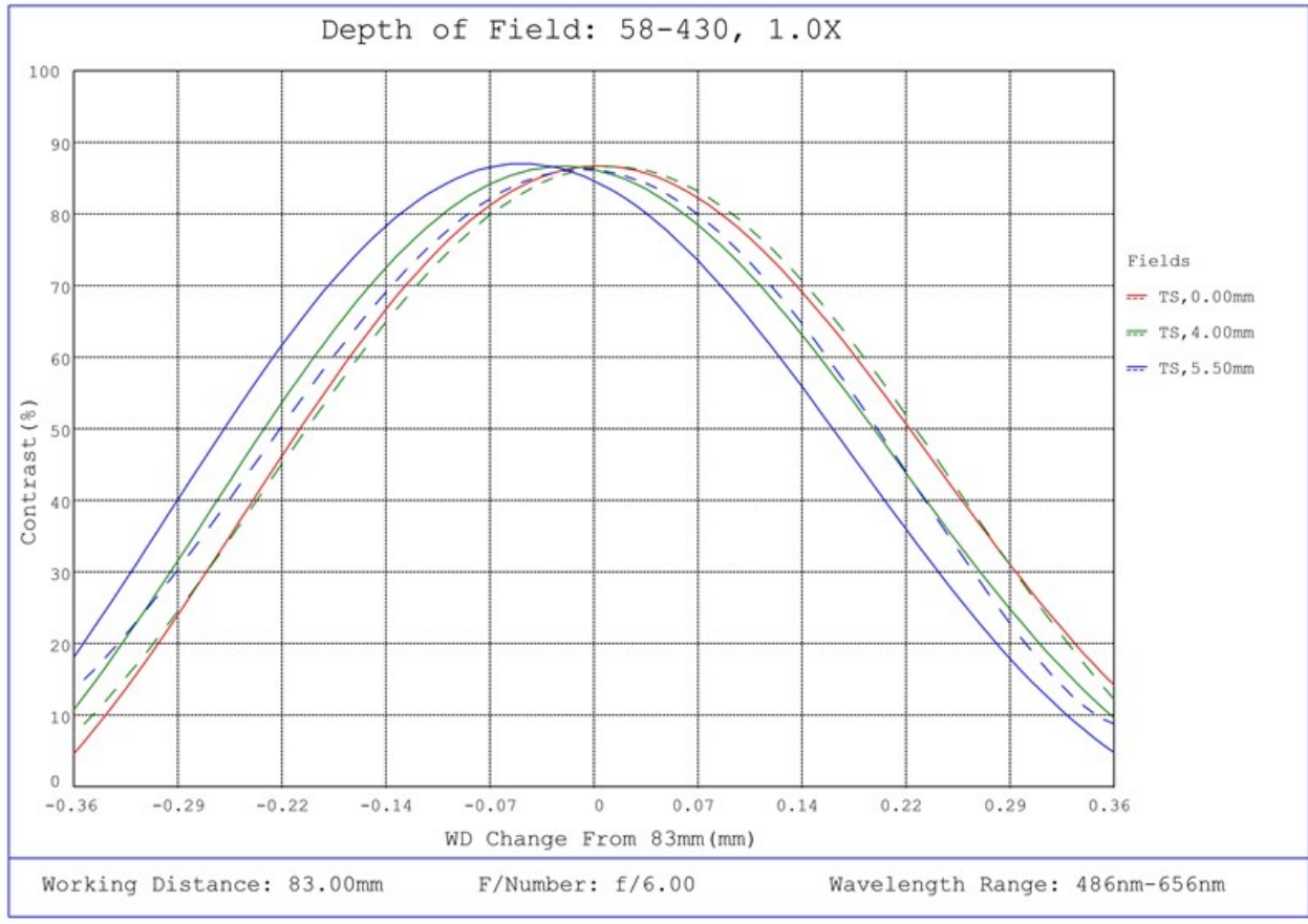
#58-430, 1.0X SilverTL™ Telecentric Lens, Depth of Field Plot, 83mm Working Distance, f6
