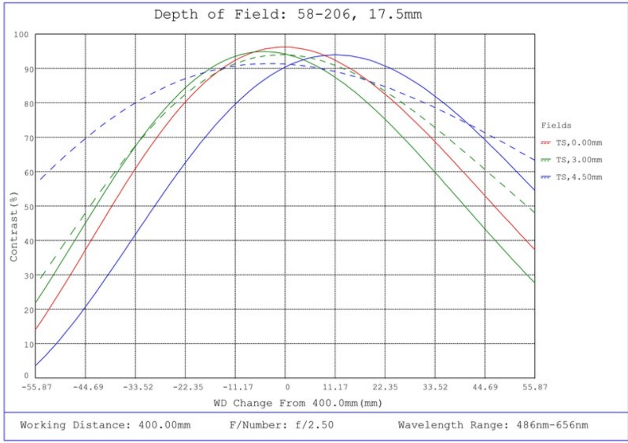
#58-206, 17.5mm FL f/2.5, Blue Series M12 Lens, Depth of Field Plot, 400mm Working Distance, f2.5
