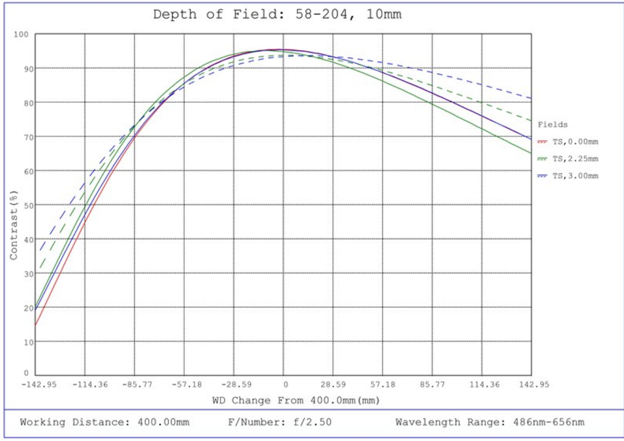
#58-204, 10mm FL f/2.5, Blue Series M12 Lens, Depth of Field Plot, 400mm Working Distance, f2.5
