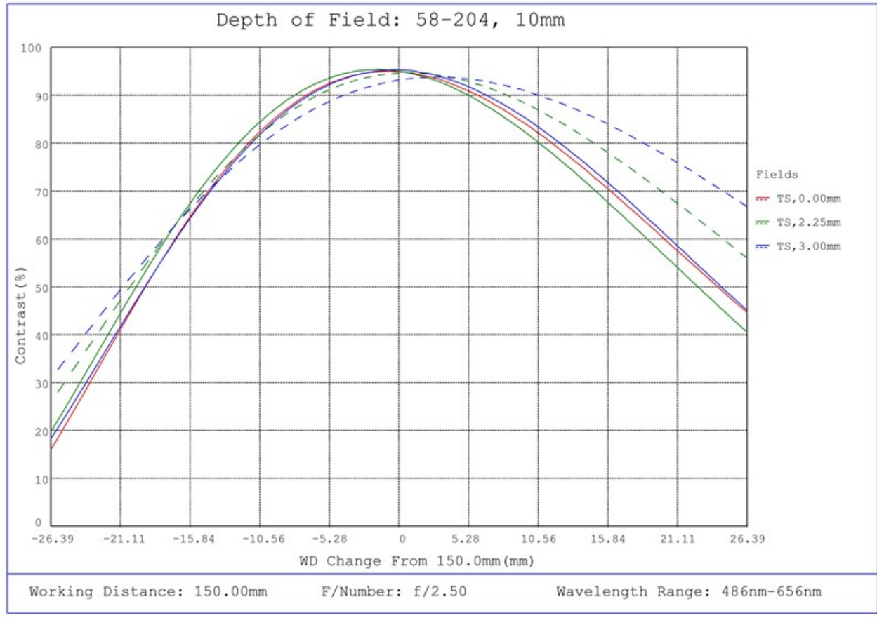
#58-204, 10mm FL f/2.5, Blue Series M12 Lens, Depth of Field Plot, 150mm Working Distance, f2.5
