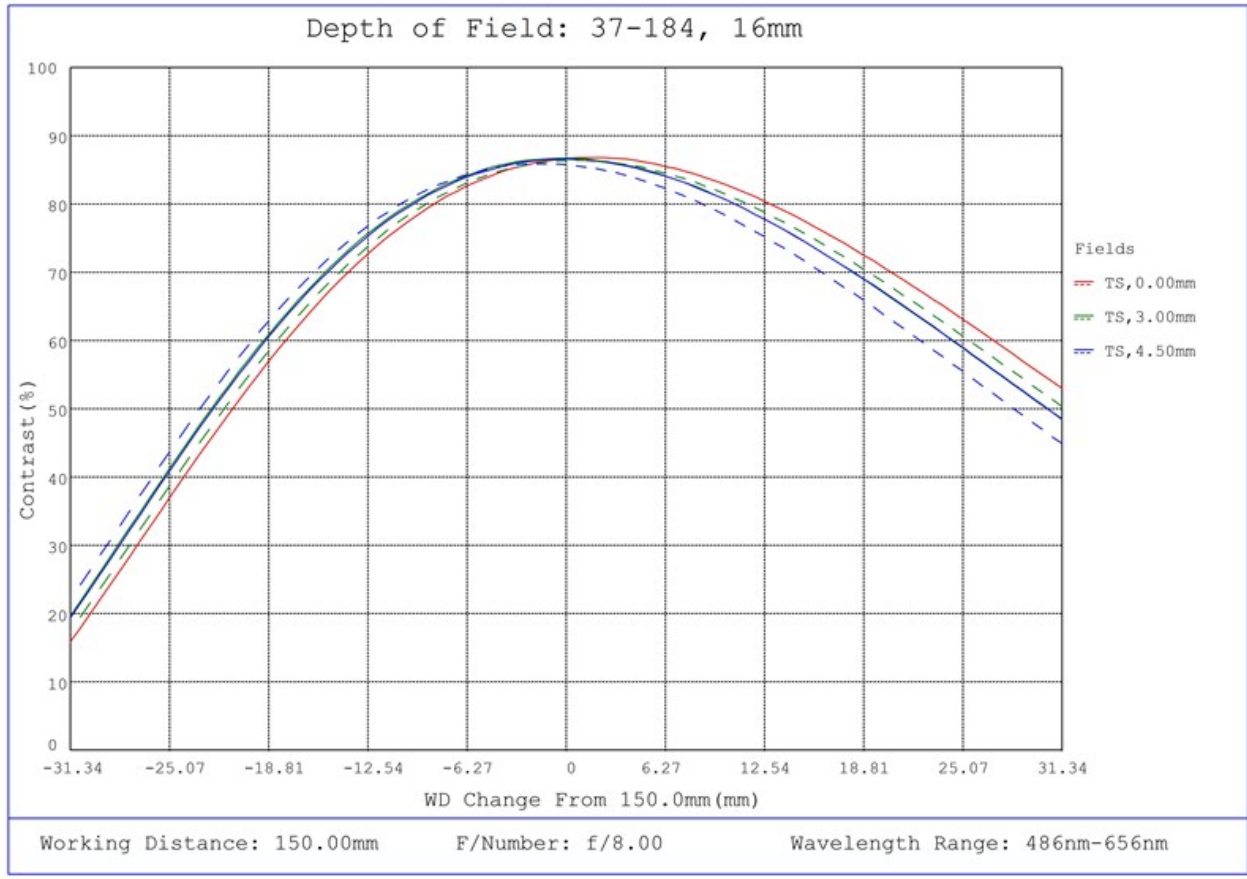
#37-184, 16mm FL f/8.0 Blue Series M12 Lens, Depth of Field Plot, 150mm Working Distance, f8
