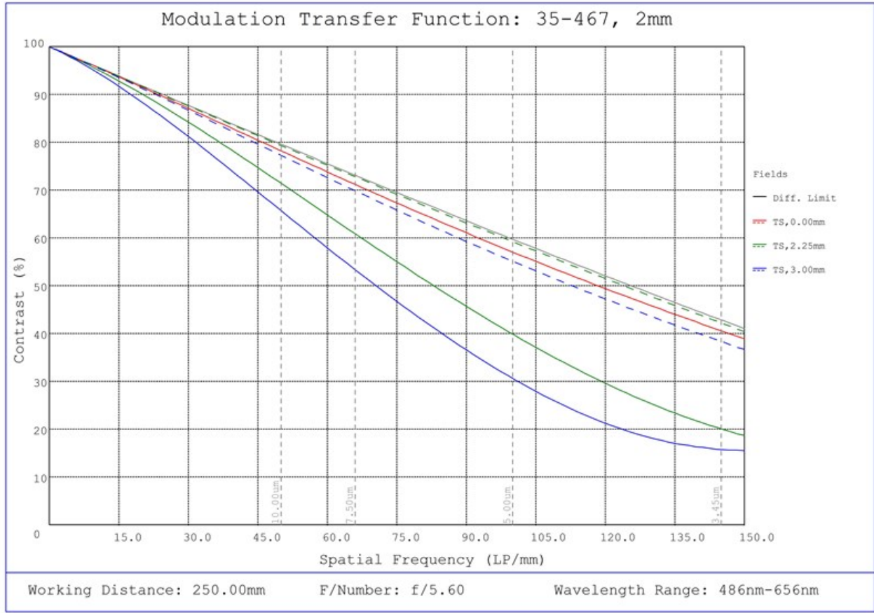
#35-467, 2mm FL f/5.6 IR-Cut, Blue Series M12 Lens, Modulated Transfer Function (MTF) Plot, 250mm Working Distance, f5.6
