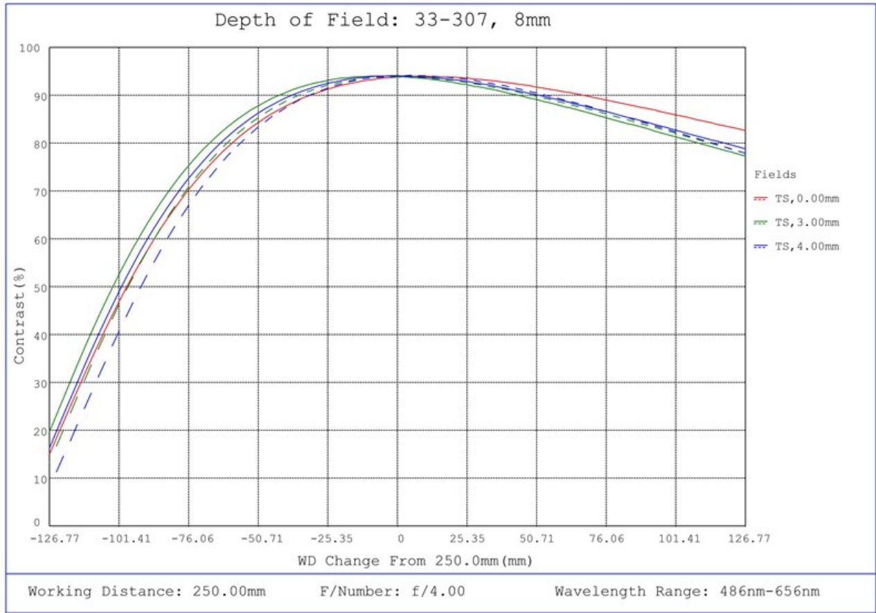
#33-307, 8mm UC Series Fixed Focal Length Lens, Depth of Field Plot, 250mm Working Distance, f4
