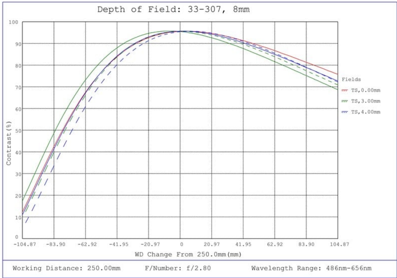
#33-307, 8mm UC Series Fixed Focal Length Lens, Depth of Field Plot, 250mm Working Distance, f2.8
