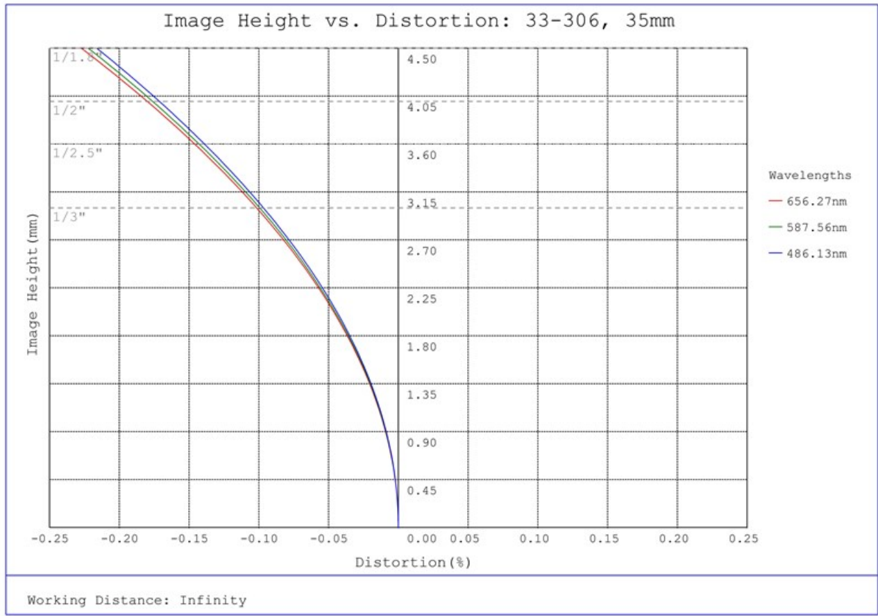
#33-306, 35mm UC Series Fixed Focal Length Lens, Distortion Plot
