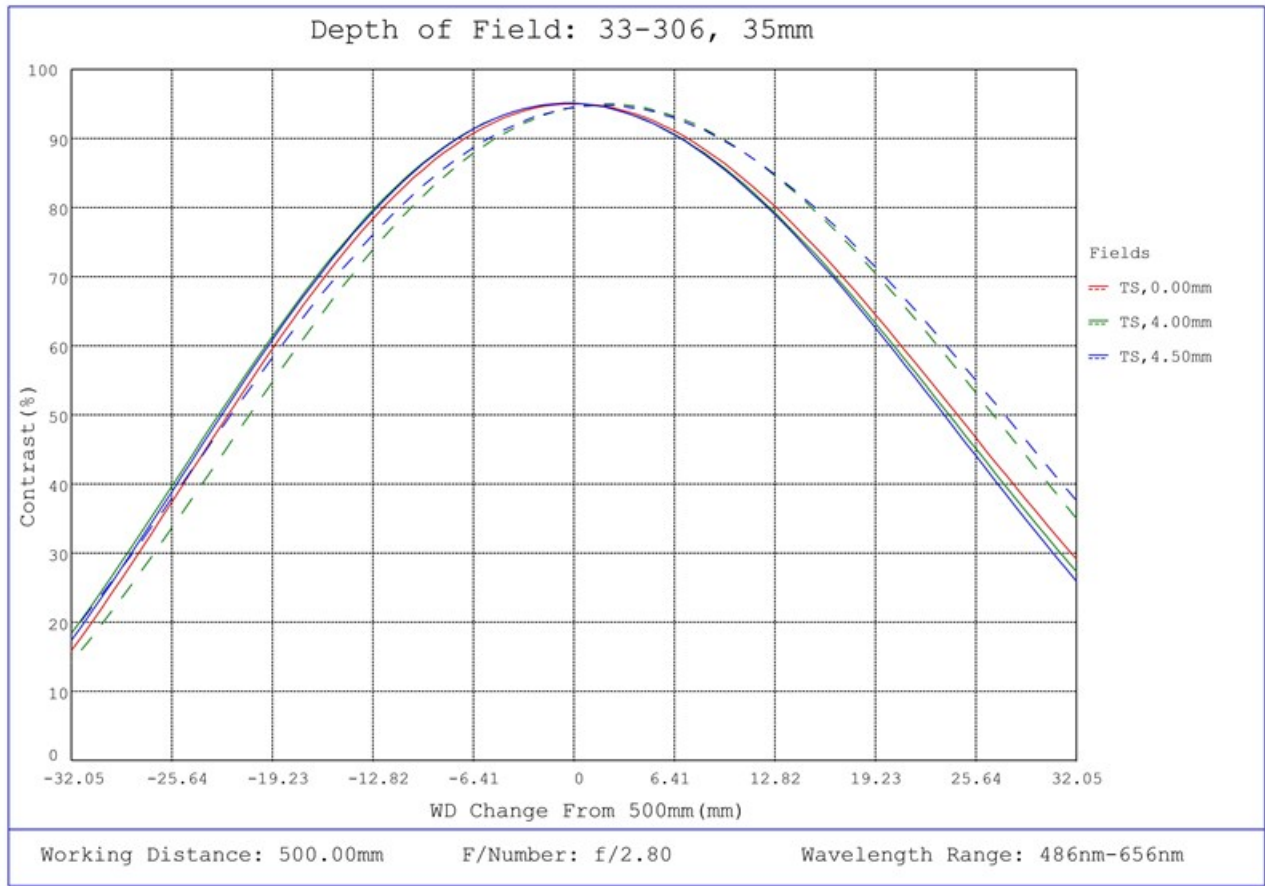
#33-306, 35mm UC Series Fixed Focal Length Lens, Depth of Field Plot, 500mm Working Distance, f2.8
