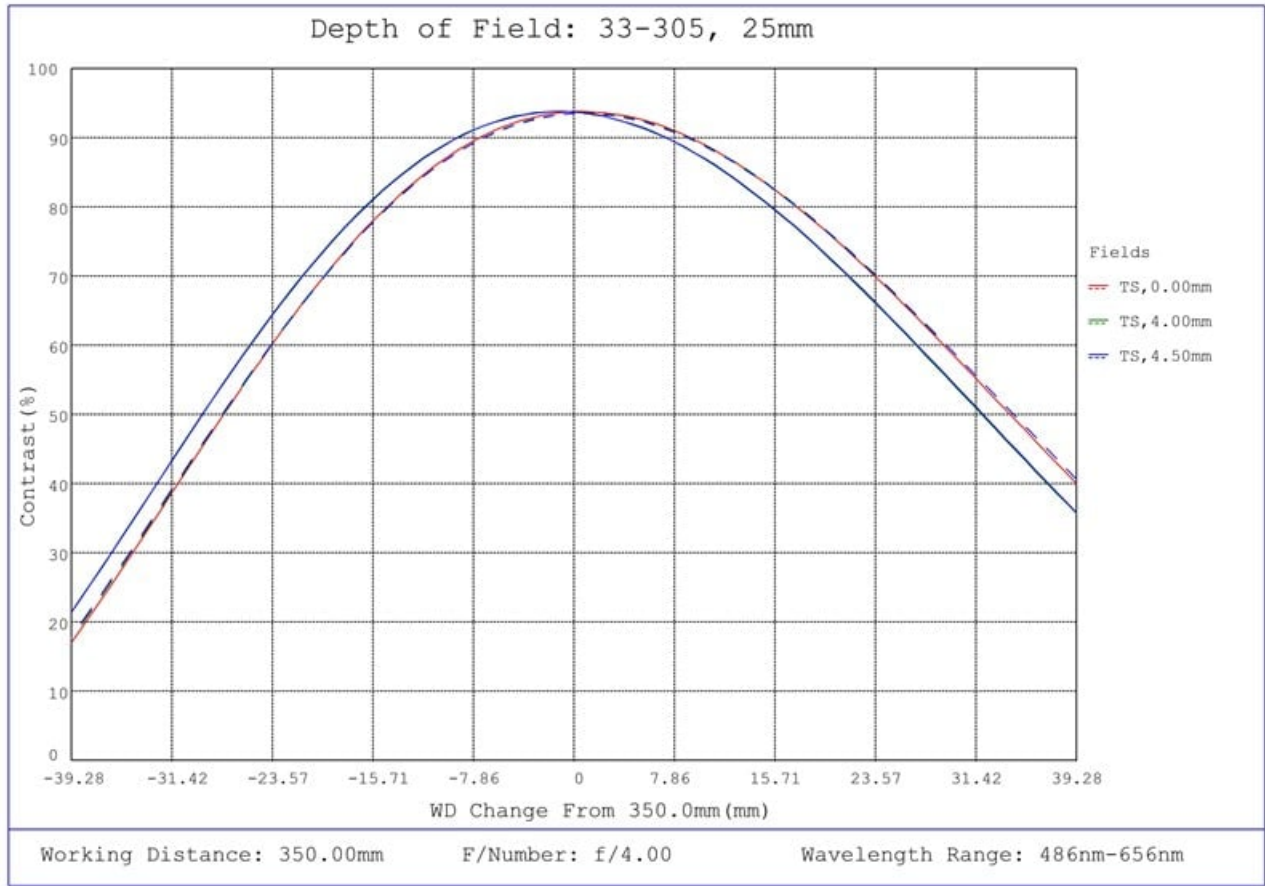
#33-305, 25mm UC Series Fixed Focal Length Lens, Depth of Field Plot, 350mm Working Distance, f4
