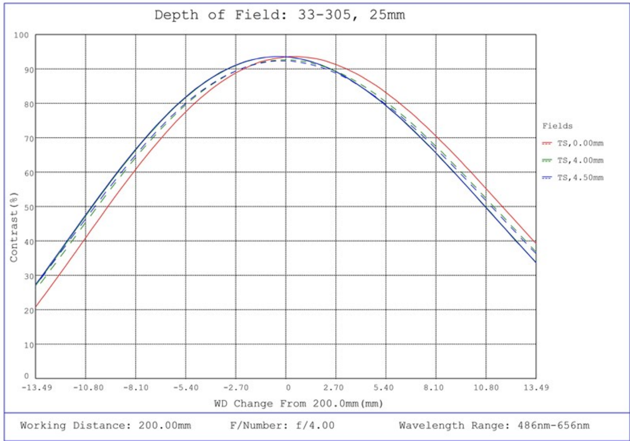
#33-305, 25mm UC Series Fixed Focal Length Lens, Depth of Field Plot, 200mm Working Distance, f4
