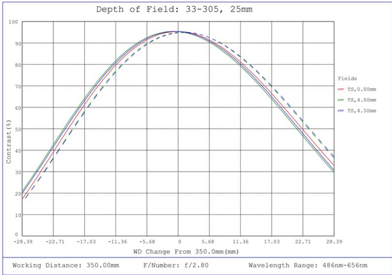
#33-305, 25mm UC Series Fixed Focal Length Lens, Depth of Field Plot, 350mm Working Distance, f2.8
