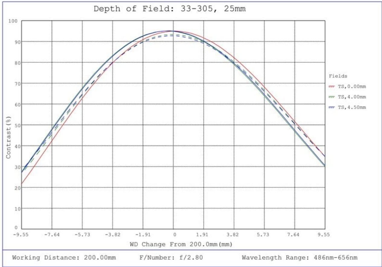
#33-305, 25mm UC Series Fixed Focal Length Lens, Depth of Field Plot, 200mm Working Distance, f2.8
