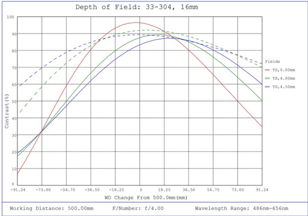
#33-304, 16mm UC Series Fixed Focal Length Lens, Depth of Field Plot, 500mm Working Distance, f4
