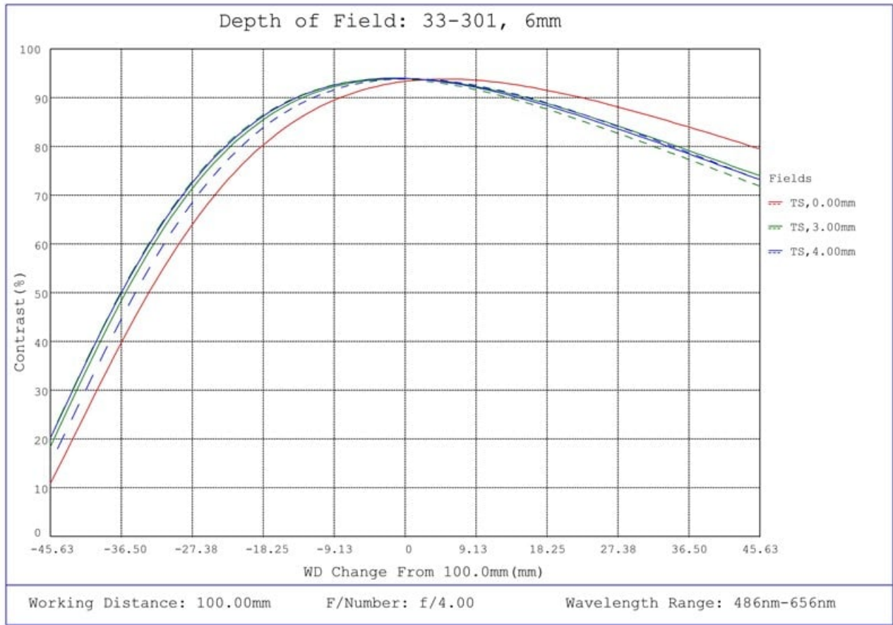
#33-301, 6mm UC Series Fixed Focal Length Lens, Depth of Field Plot, 100mm Working Distance, f4
