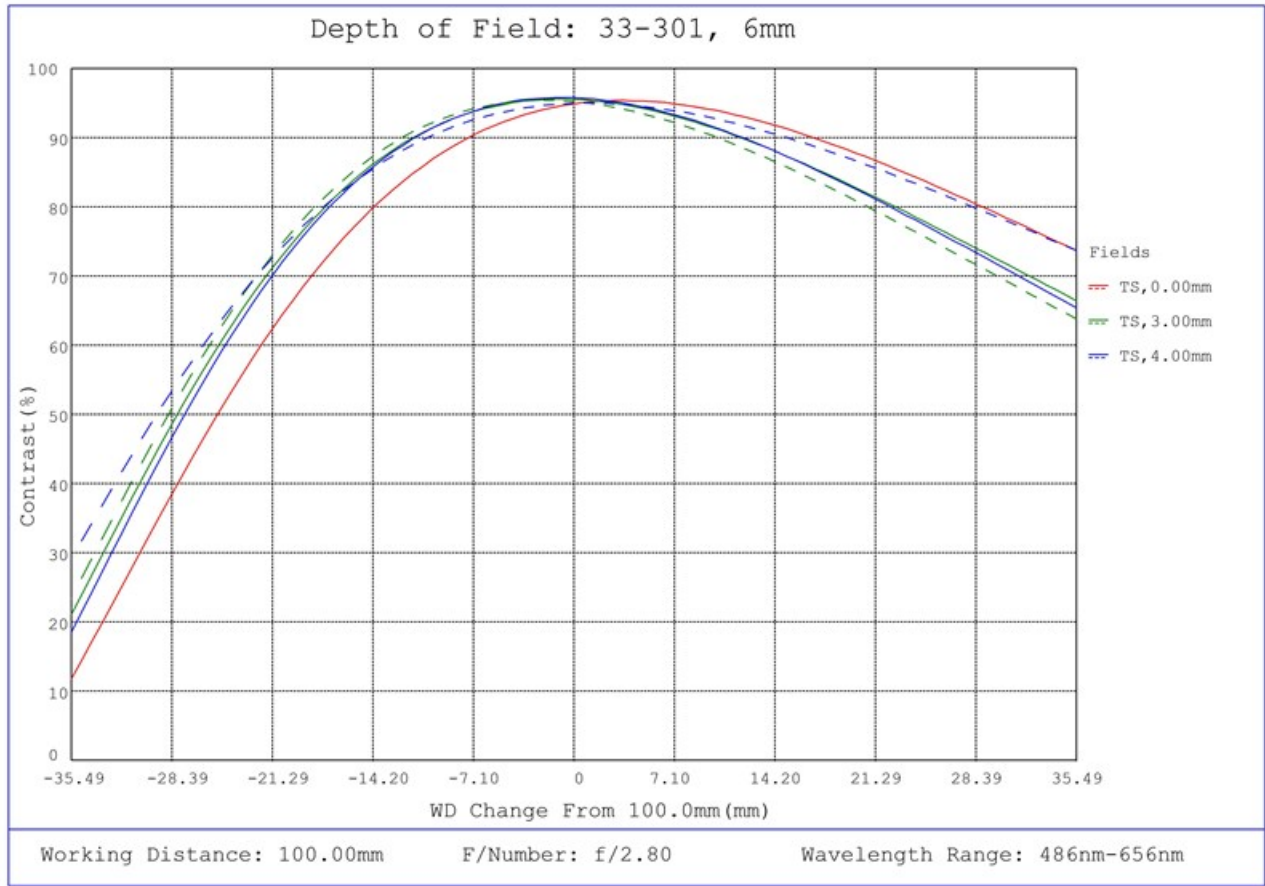
#33-301, 6mm UC Series Fixed Focal Length Lens, Depth of Field Plot, 100mm Working Distance, f2.8
