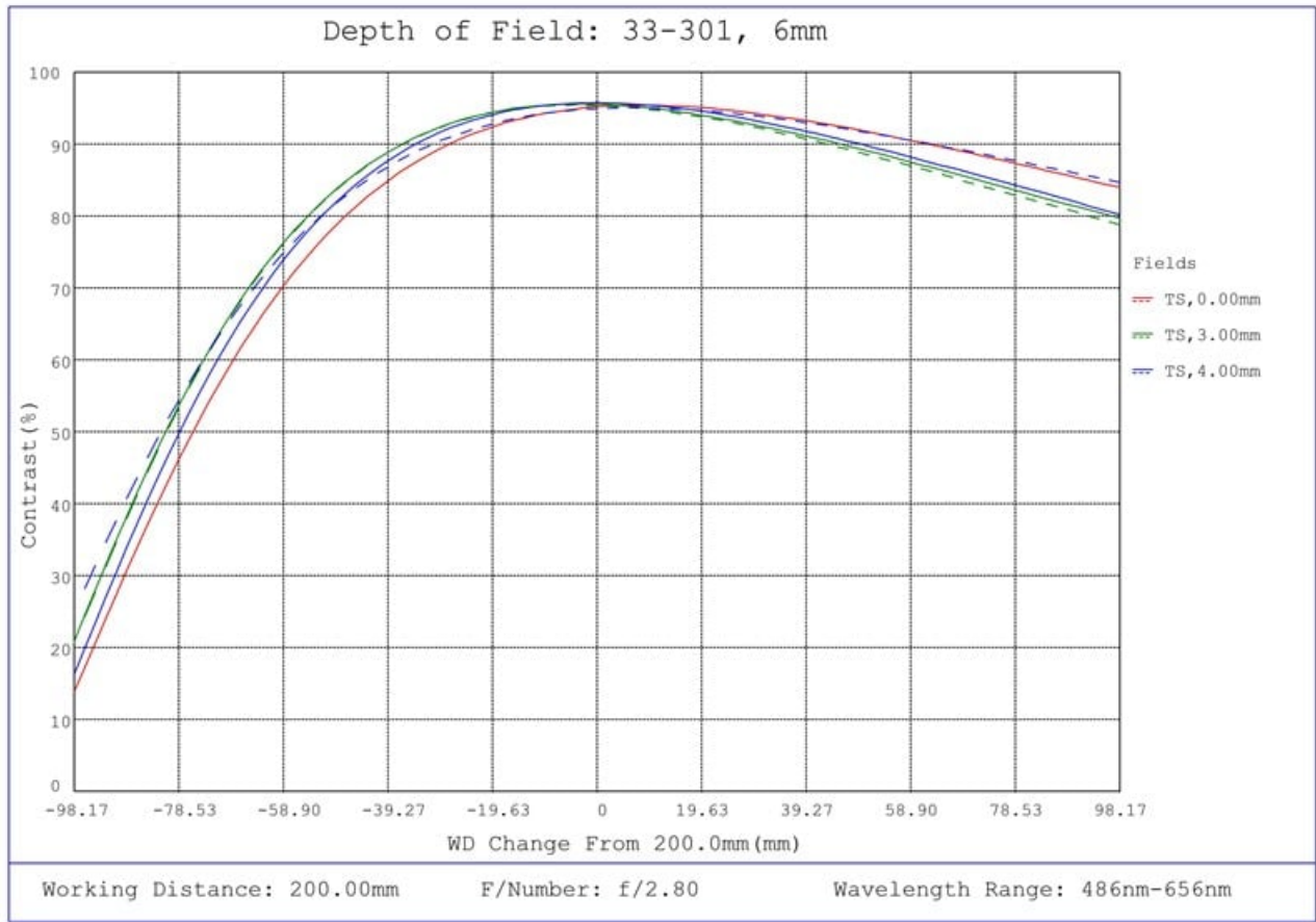
#33-301, 6mm UC Series Fixed Focal Length Lens, Depth of Field Plot, 200mm Working Distance, f2.8
