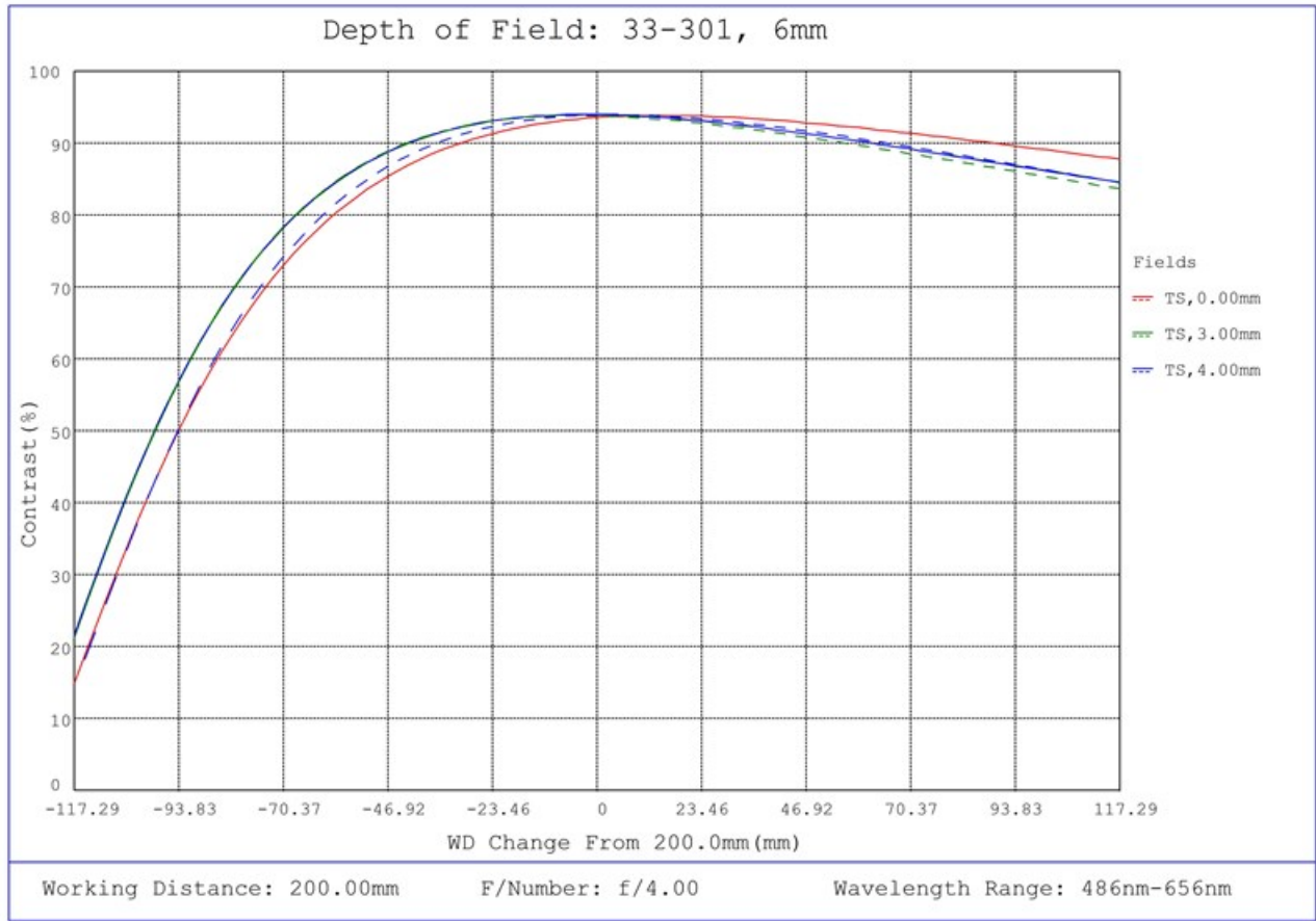
#33-301, 6mm UC Series Fixed Focal Length Lens, Depth of Field Plot, 200mm Working Distance, f4
