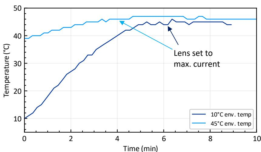
Figure 6: Initial heating phase for two extreme environmental temperatures 10°C and 40°C.
