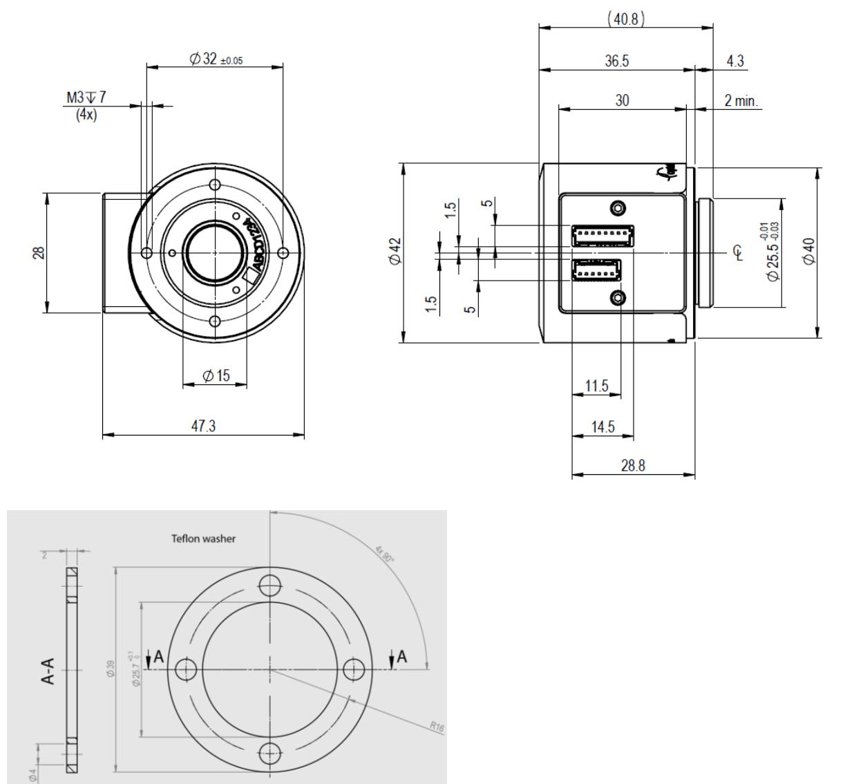
Figure 1: Mechanical layout of the EL-10-42-OF (units: mm). Four M3 thread holes are available four mounting. The Teflon washer has a thickness of 2mm with a flatness tolerance of +/- 0.05 mm.
