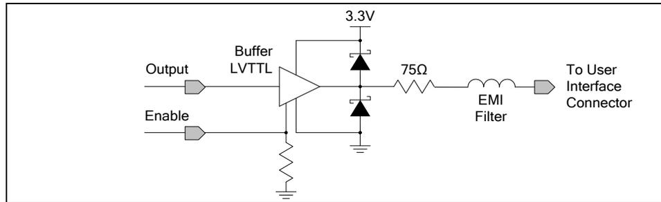
Figure 29: General Outputs Electrical Diagram
