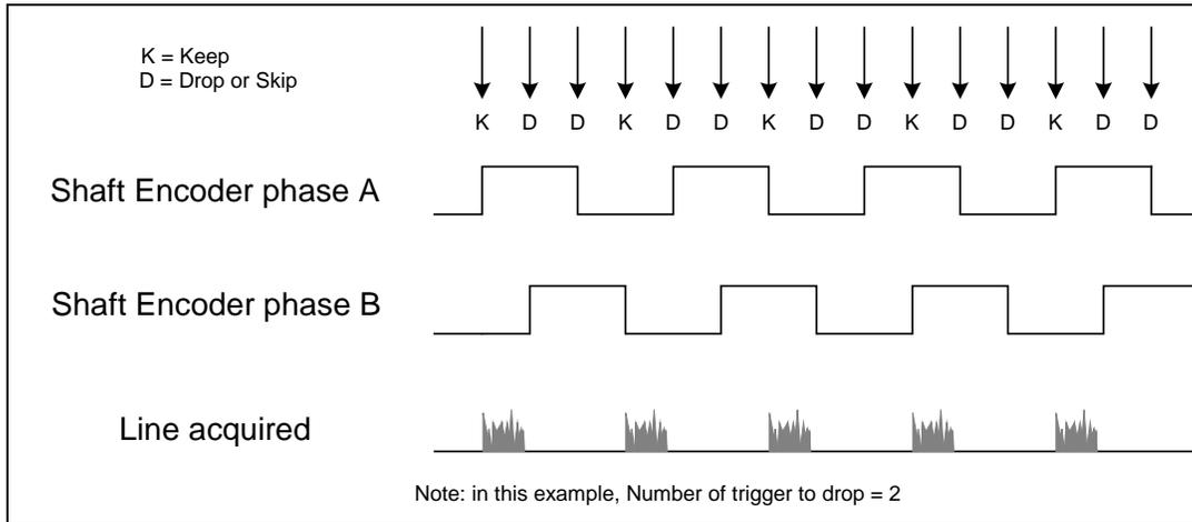
Figure 13: Encoder Input with Pulse-drop Counter
