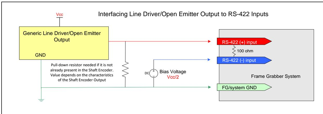
Figure 34: Interfacing to a Line Driver Output
