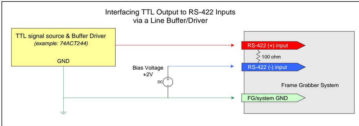
Figure 33: Interfacing TTL to RS-422 Shaft Encoder Inputs
