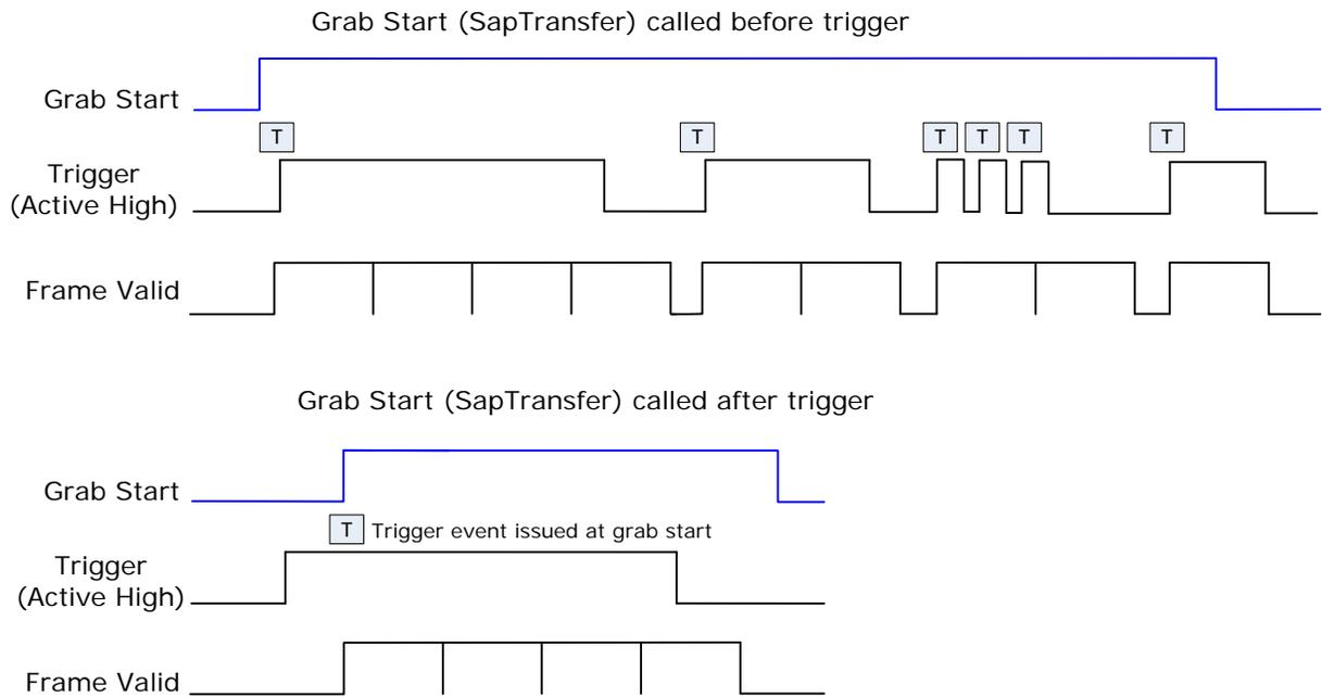
Figure 18: Line scan, Fixed Frame, Level Trigger (Roll-Over to Next Frame)
