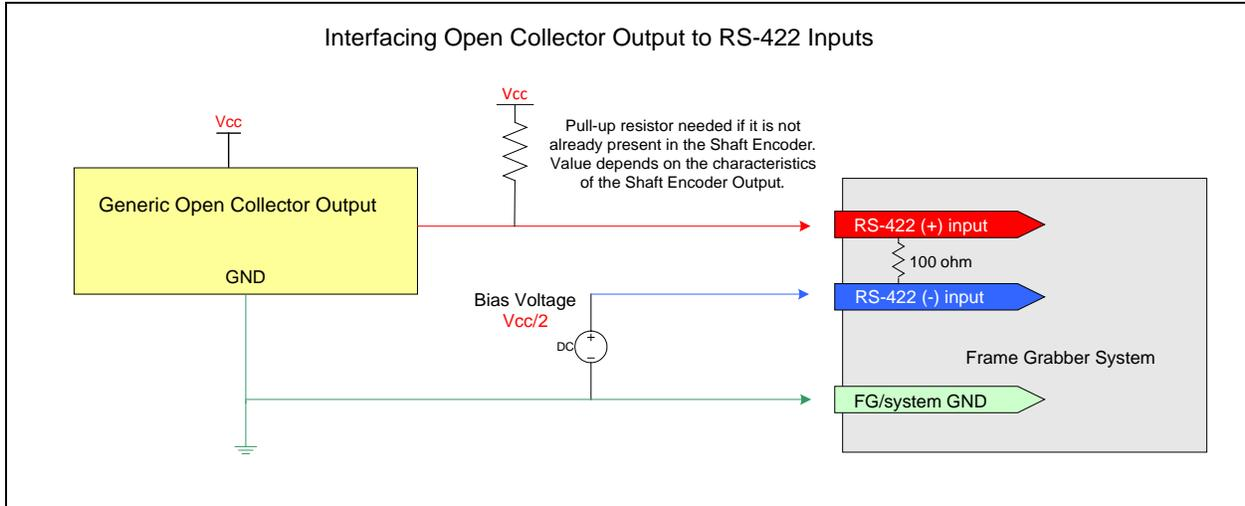
Figure 35: Interfacing to an Open Collector Output
