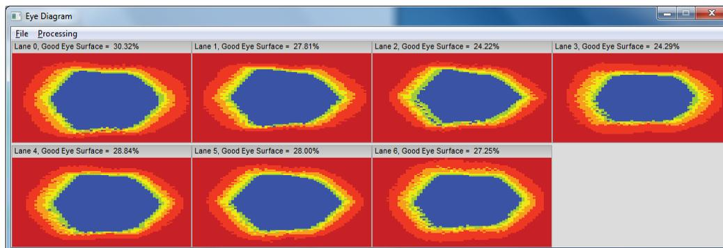
Figure 44: Diagnostic Tool Eye Diagram
