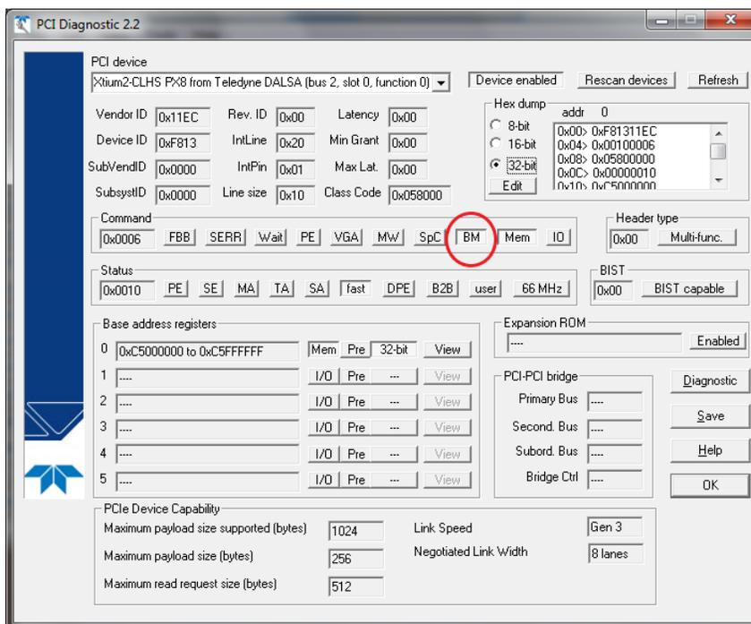
Figure 49: PCI Diagnostic Tool BM Button
