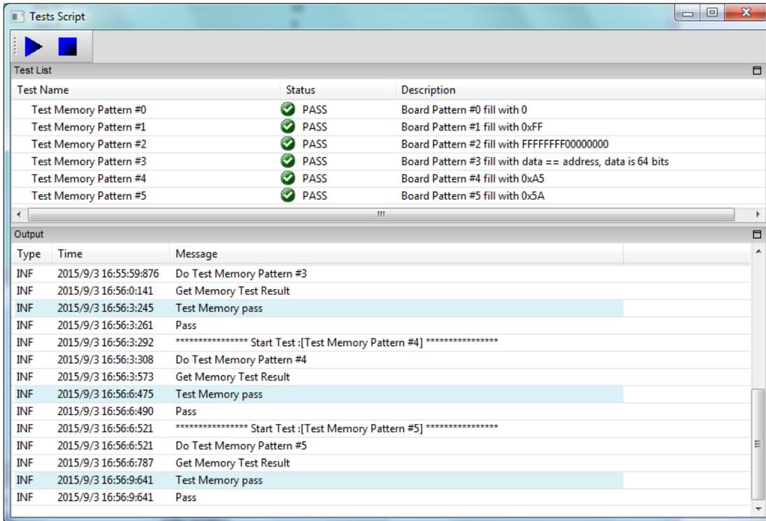
Figure 43: Diagnostic Tool Self-Test Window
