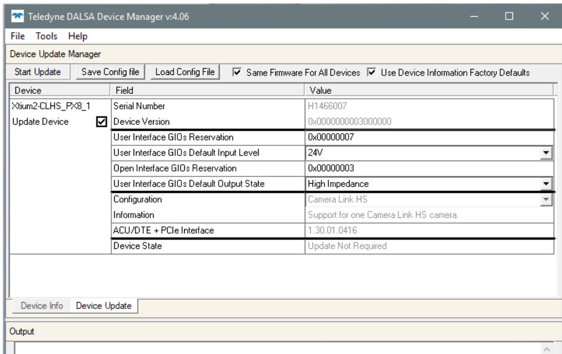
Figure 48: Board Firmware Version
