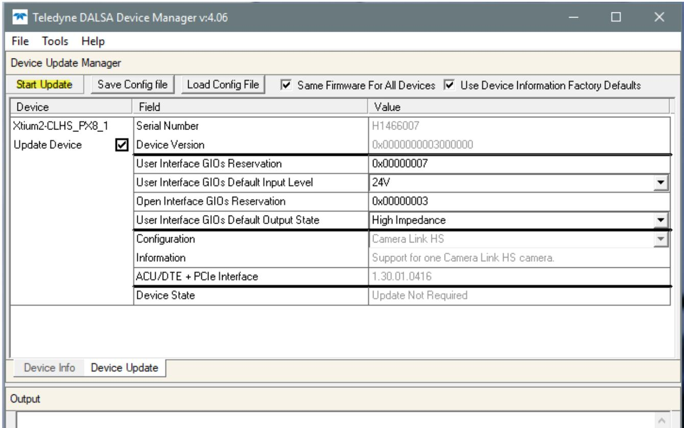
Figure 4: Device Manager Parameter Setting Differences
