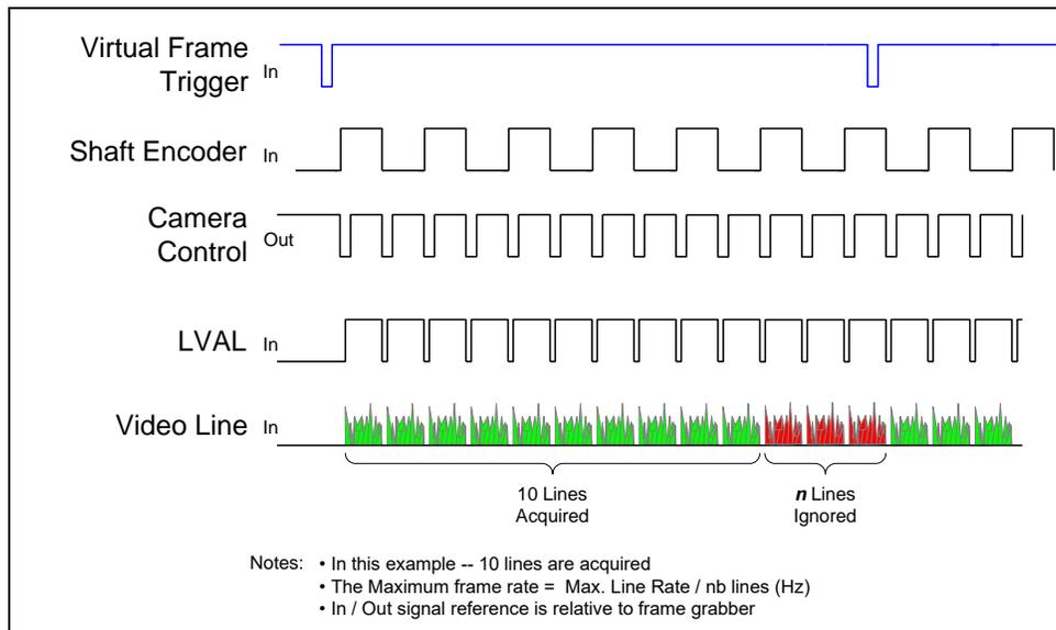
Figure 15: Synchronization Signals for a 10 Line Virtual Frame
