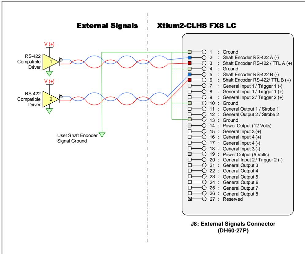
Figure 32: External RS-422 Signals Connection Diagram
