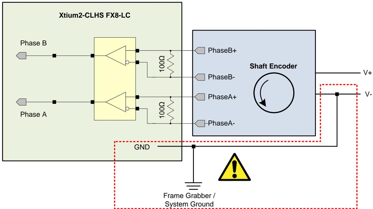
Figure 31: RS-422 Shaft Encoder Input Electrical Diagram
