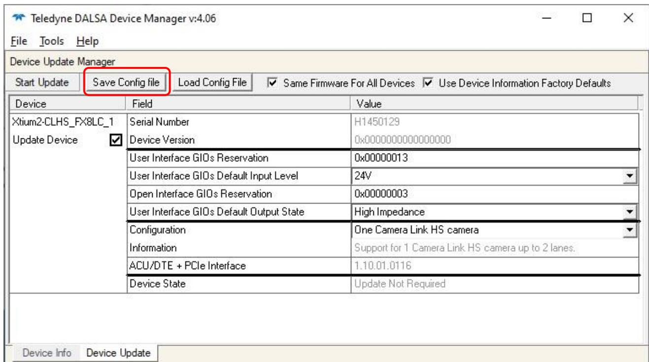
Figure 41: Create an install.ini File
