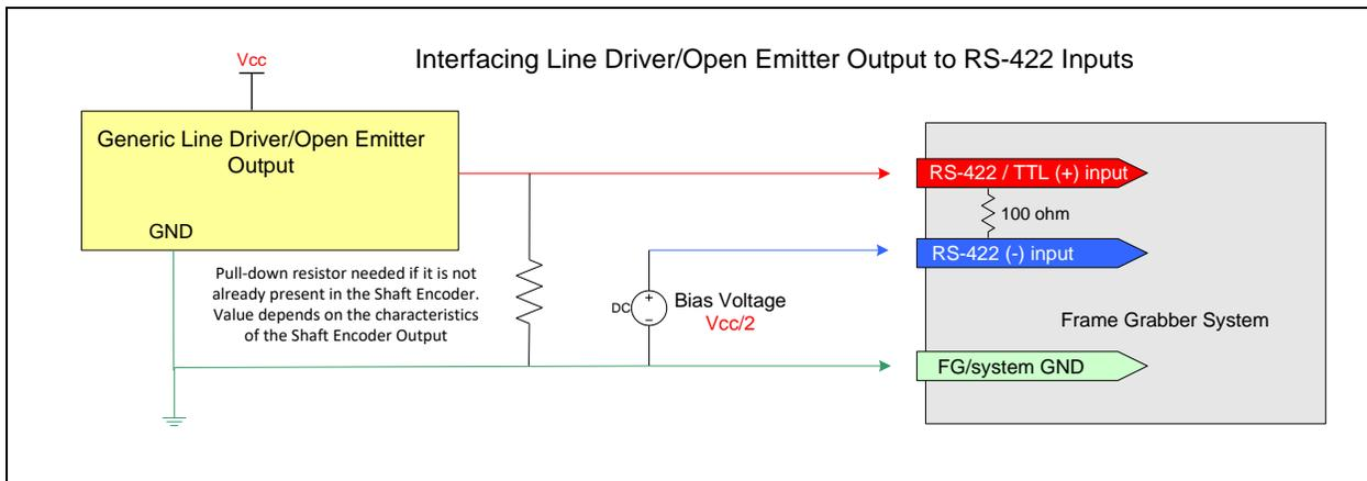
Figure 33: Interfacing to a Line Driver Output
