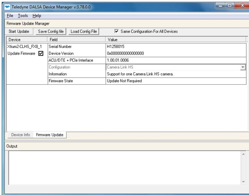
Figure 49: Board Firmware Version
