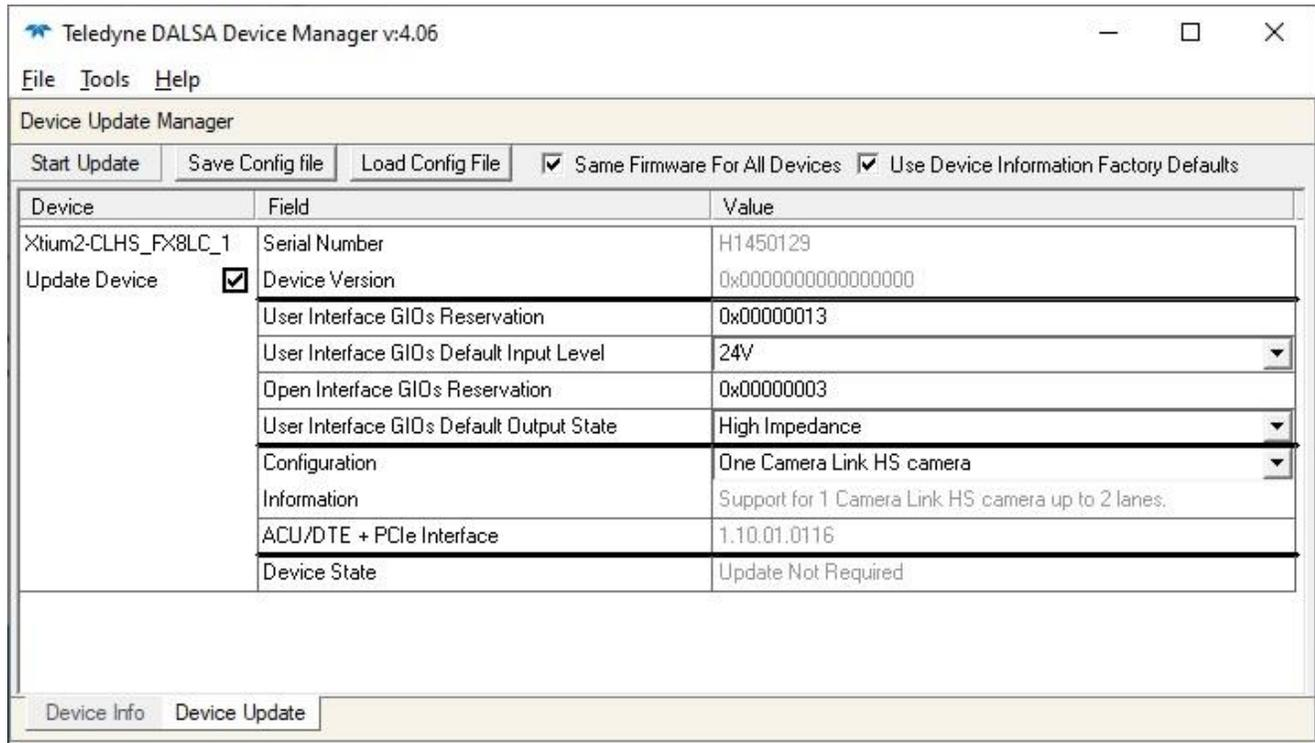
Figure 4: Device Manager Parameter Setting Differences
