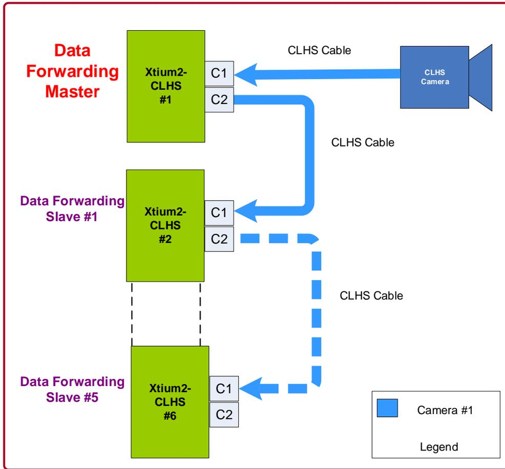
Figure 25: Data Forwarding using a single camera of 1 lane Block Diagram
