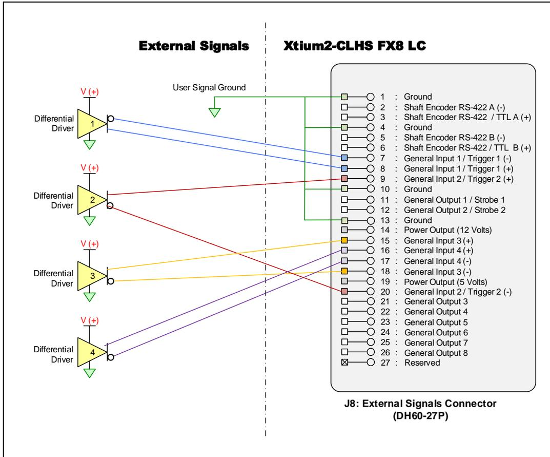
Figure 28: External Signals Connection Diagram
