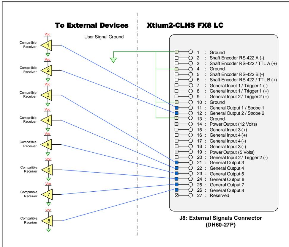
Figure 30: Output Signals Connection Diagram
