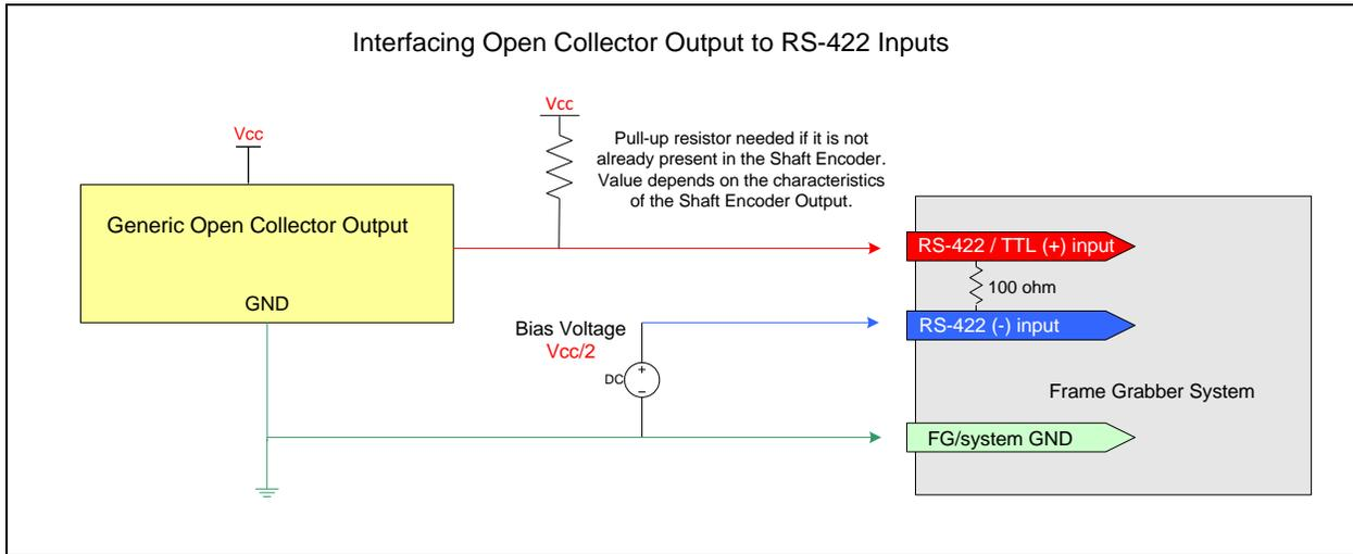
Figure 34: Interfacing to an Open Collector Output
