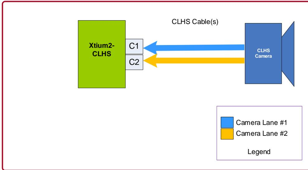
Figure 23: One Camera up to 2 lanes Block Diagram
