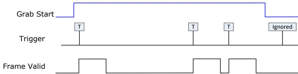
Figure 17: Line scan, Fixed Frame, Edge Trigger
