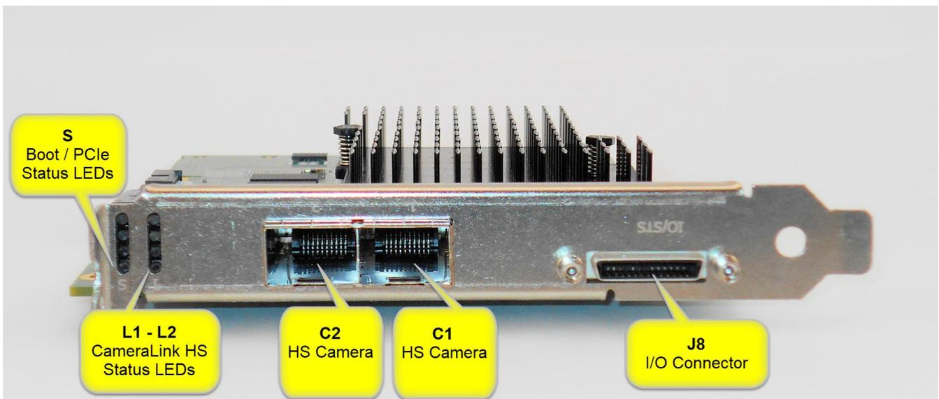
Figure 22: End Bracket Details
