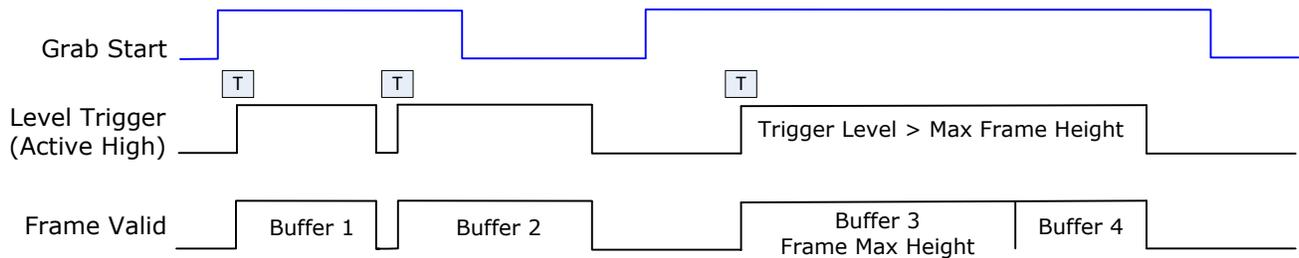
Figure 20: Line scan, Fixed Frame, Level Trigger (Roll-Over)
