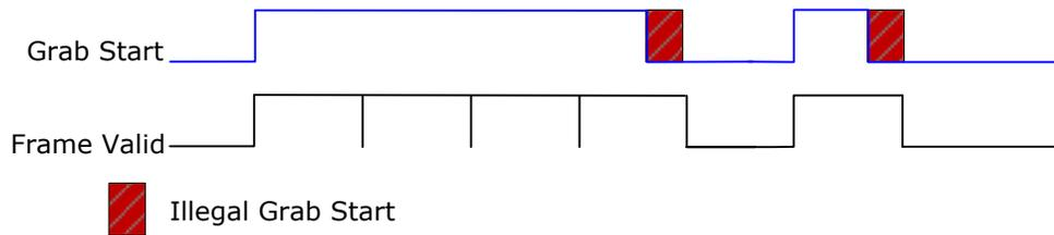
Figure 16: Line scan, Fixed Frame, No Trigger
