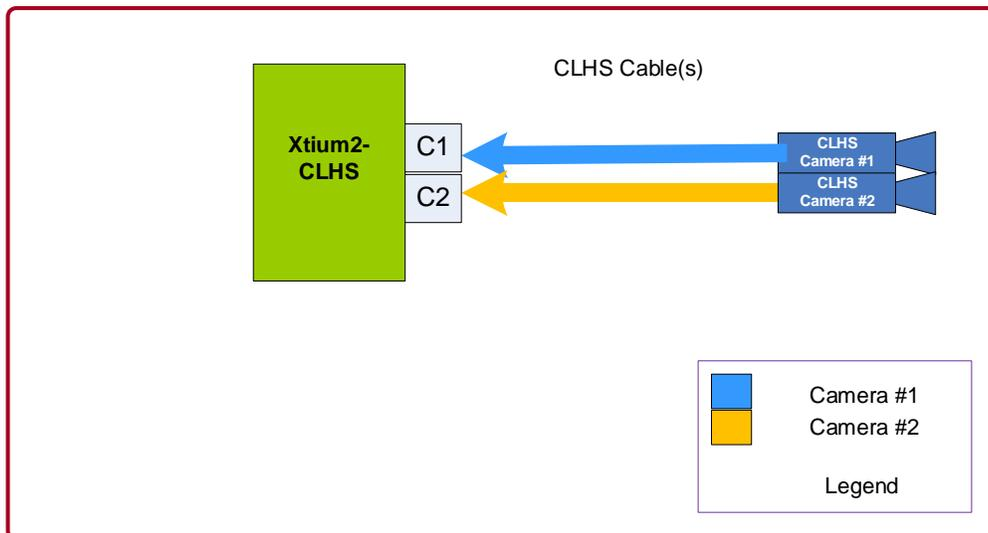
Figure 24: Dual Camera of 1 lane each Block Diagram
