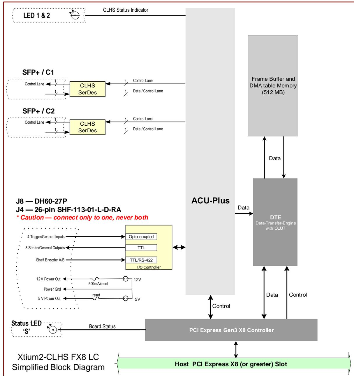
Figure 10: Xtium2-CLHS FX8 LC Block Diagram
