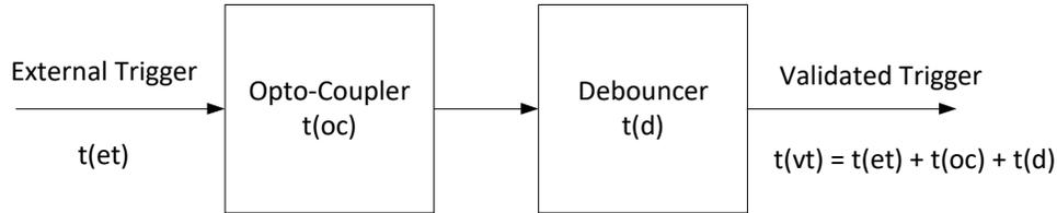
Figure 27: External Trigger Input Validation & Delay
