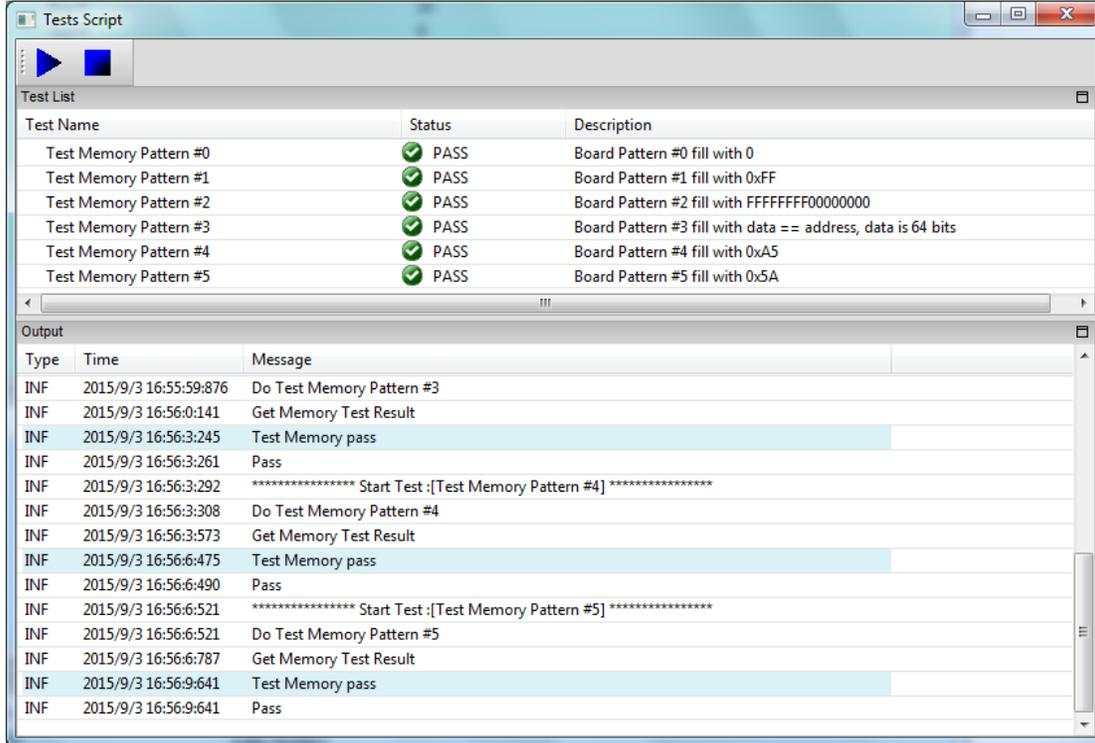
Figure 44: Diagnostic Tool Self-Test Window
