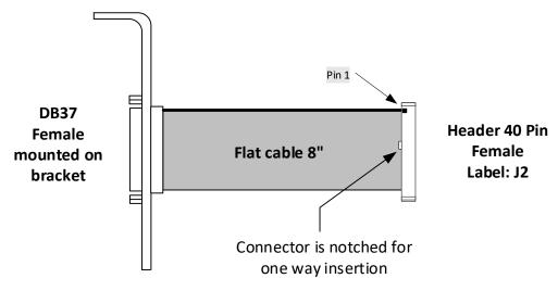
Figure 47: DB37 Output Cable
