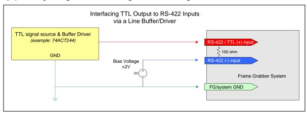
Figure 42: Interfacing TTL to RS-422 Shaft Encoder Inputs using a Bias Voltage
