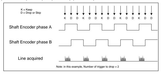
Figure 18: Encoder Input with Pulse-drop Counter
