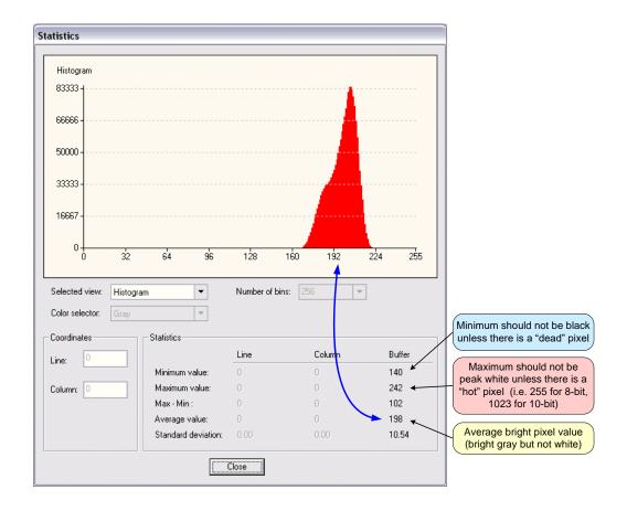
**Important:** In this example, the **average** pixel value for the frame is bright gray. Also note that sensors may show a much higher maximum or a much lower minimum pixel value due to one or more "hot or dead pixels". The sensor specification accounts for a small number of hot, stuck, or dead pixels (pixels that do not react to light over the full dynamic range specified for that sensor).
