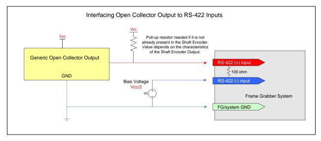
Figure 40: Interfacing to an Open Collector Output
