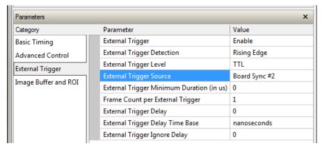
• **Test Setup:** Start the acquisition on all slave boards. The acquisition process is now waiting for the control signal from the master board. Trigger master board acquisition and the acquisition start signal is sent to each slave board.
