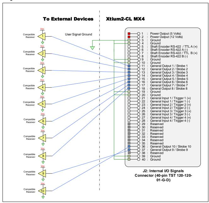
Figure 35: Output Signals to J2 Connection Diagram
