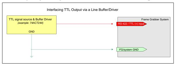
Figure 41: Interfacing TTL to TTL Shaft Encoder Inputs
