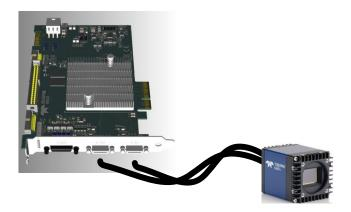
If using PoCL, use CamExpert to enable the PoCL feature in the Basic Timing category.
