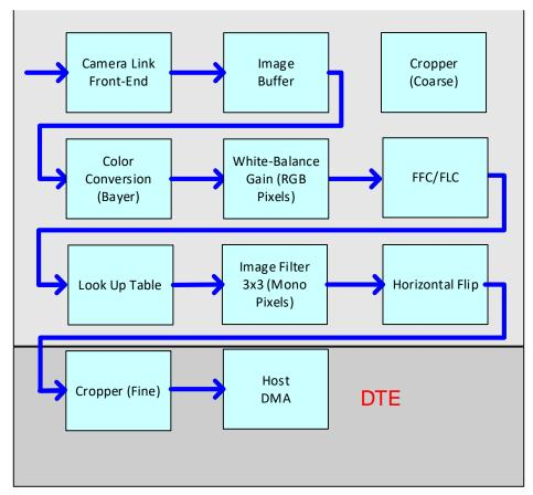
Figure 16: Xtium2-CL MX4 Flow Diagram
