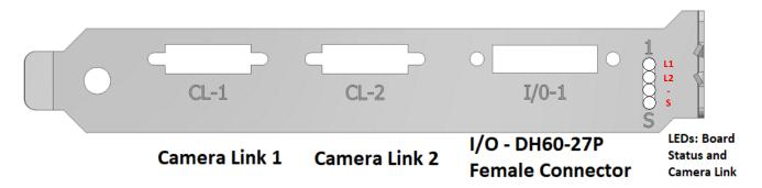
Figure 27: End Bracket Details
