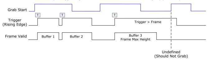
Figure 24: Line scan, Variable Frame, Edge Trigger (Active High determines Frame Length)
