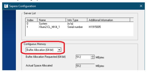
Adjust this value higher if your application generates any out-of-memory error while allocating host frame buffers or when connecting the buffers via a transfer object. You can approximate the worst-case scenario amount of contiguous memory required as follows:
