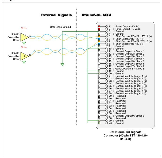
Figure 38: External RS-422 Signals to J2 Connection Diagram
