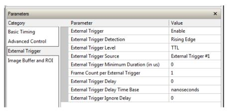
The Sync Master Xtium2 board is also configured to output the external trigger on board sync #1, as shown in the following image.
