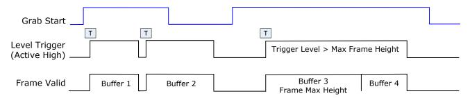
Figure 25: Line scan, Variable Frame, Level Trigger (Roll-Over)
