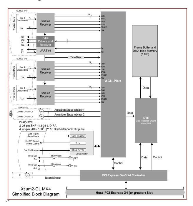
Figure 15: Xtium2-CL MX4 Model Block Diagram
