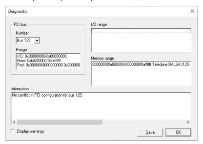
Figure 55: PCI Diagnostic Program – PCI bus info
