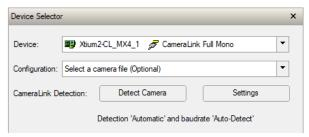
If the Detect Camera button is disabled, click Settings to open the the Communication Settings dialog to configure CamExpert to detect attached cameras using a serial port.
