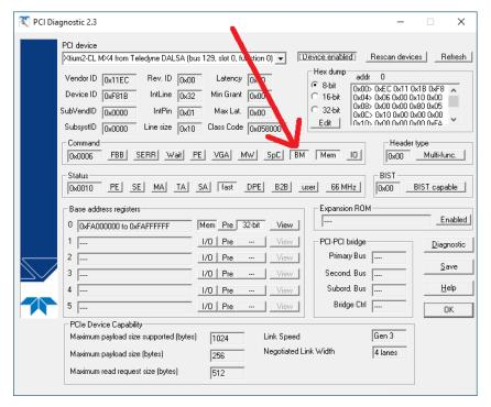
Figure 58: PCI Diagnostic – checking the BUS Master bit
