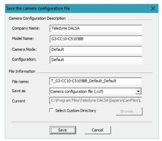
The Xtium2-CL MX4 can be configured using the the parameter settings in this file when using the Sapera LT API in your application to acquire images
