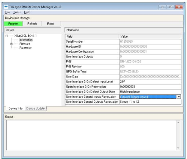
When programming is complete, the Reset button is displayed in green, click the button to reset the board.
