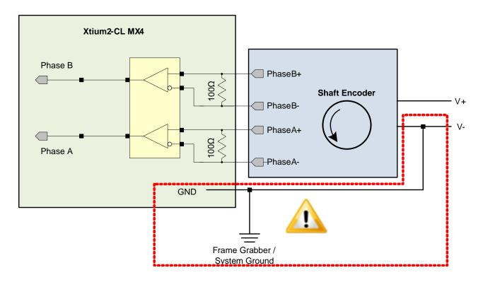
Figure 36: RS-422 Shaft Encoder Input Electrical Diagram
