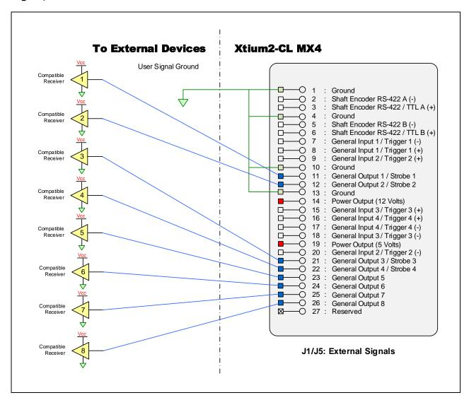
Figure 34: Output Signals to J1/J5 Connection Diagram
