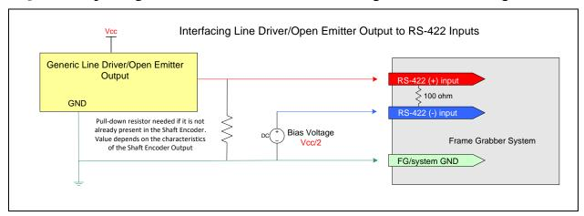
Figure 39: Interfacing to a Line Driver Output
