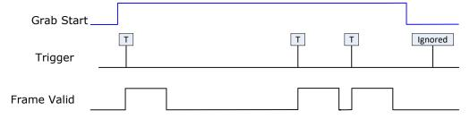
Figure 22: Line scan, Fixed Frame, Edge Trigger
