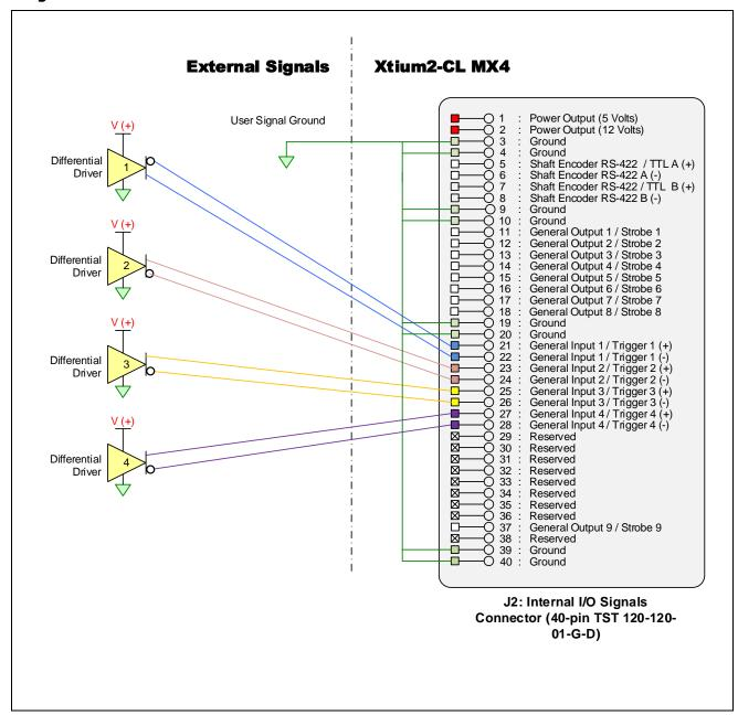
Figure 32: External Signals to J2 Connection Diagram
