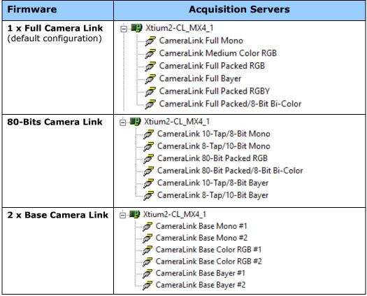
Depending on the selected server, different parameters may be displayed. For example, with an RGB acquisition server, the Color Type parameter is not displayed since its value is not configurable. For more information, see the Sapera Servers & Resources section.
