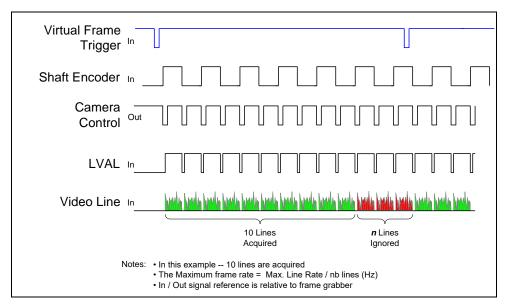
Figure 20: Synchronization Signals for a 10 Line Virtual Frame
