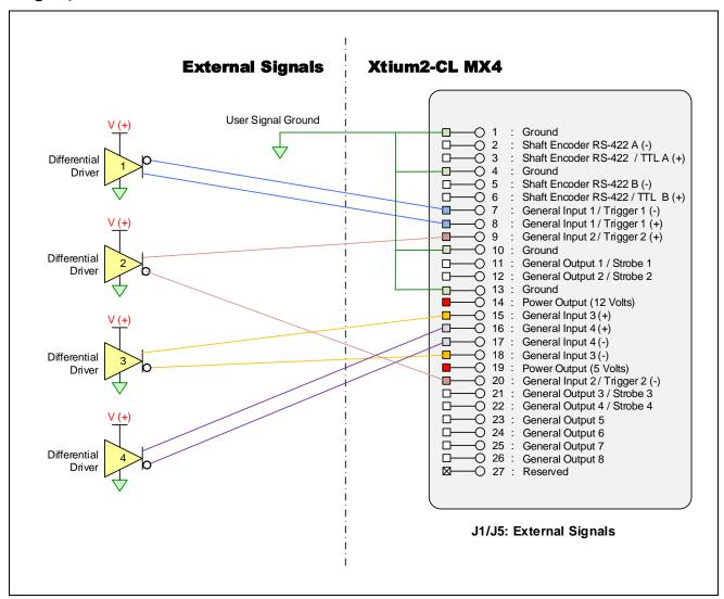
Figure 31: External Signals to J1/J5 Connection Diagram
