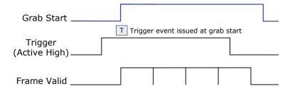
Figure 23: Line scan, Fixed Frame, Level Trigger (Roll-Over to Next Frame)
