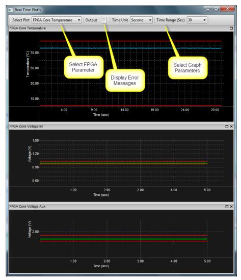
Figure 53: PCI Diagnostic Tool Live Monitoring Window
