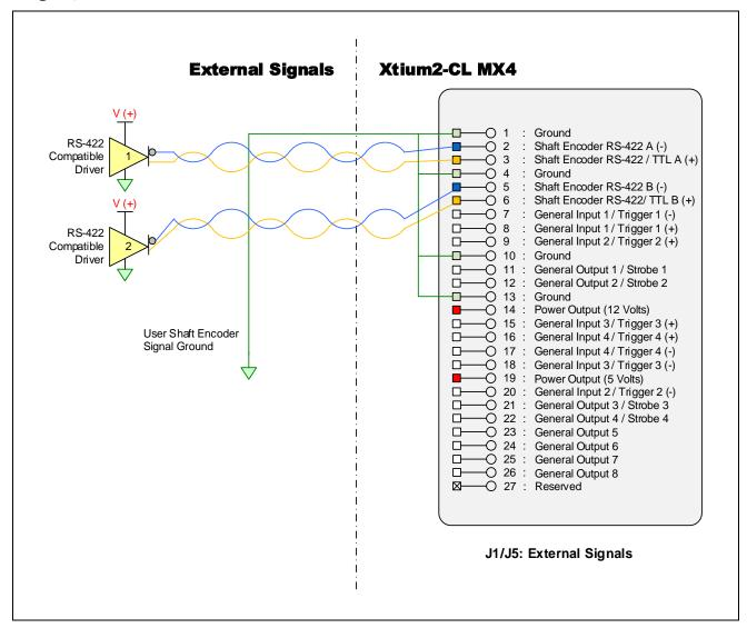
Figure 37: External RS-422 Signals to J1/J5 Connection Diagram
