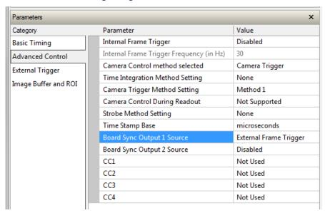
The Sync Slave Xtium2 board is configured to receive its trigger on the board sync signal. As
