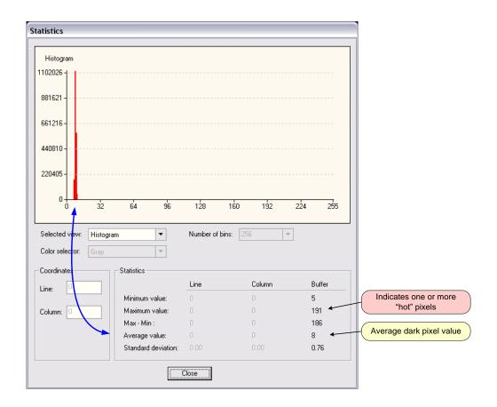
**Important:** In this example, the **average** pixel value for the frame is close to black. Also note that most sensors will show a much higher maximum pixel value due to one or more "hot pixels". The sensor specification accounts for a small number of hot or stuck pixels (pixels that do not react to light over the full dynamic range specified for that sensor).
