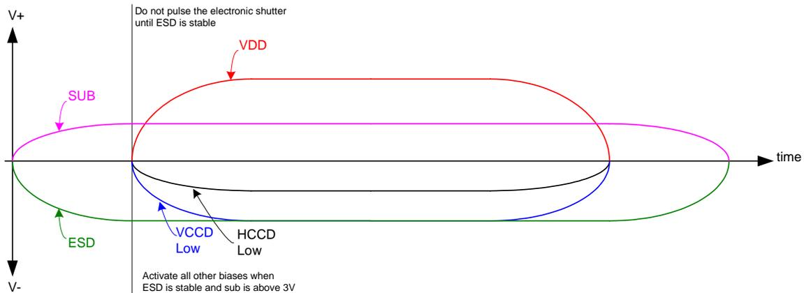
Figure 12: Power Up and Power Down Sequence
