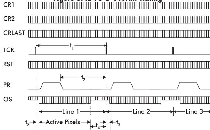
**Figure 4. IL-P3-B Detailed Readout Register Timing**
