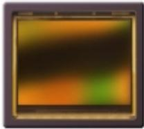
The CHR70M is a high resolution CMOS image sensor with 10000 by 7096 pixels. The image array consists of 3.1µm x 3.1µm pinned diode pixels which
