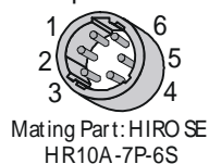
Figure 12: Hirose 6-pin Circular Male—Power Connector
