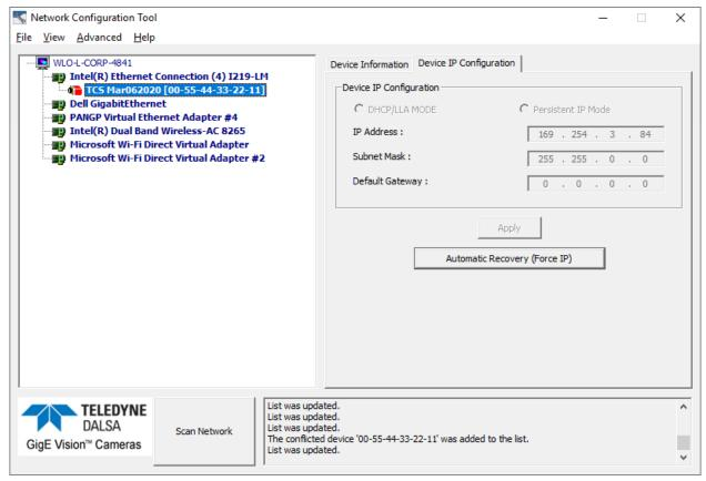
Figure 92: Network Configuration Tool – Automatic Recovery (Force IP)
