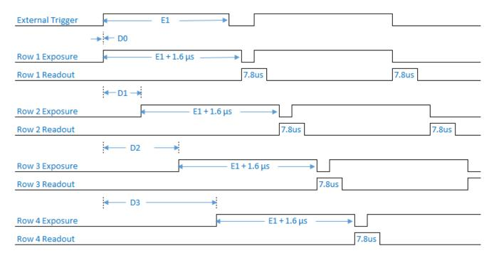
Figure 44: External Trigger Width Exposure
