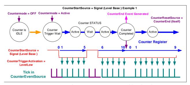
Figure 52: Example - CounterStartSource = Signal (Level Base)
