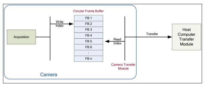
Figure 65: Transfer Control Mode
