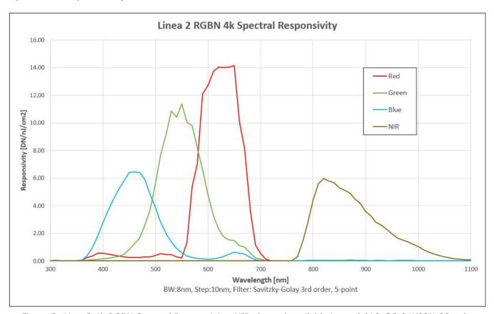
Figure 2: Linea2 4k RGBN Spectral Responsivity. NIR channel available in model L2-GC-04K03N-00 only.
