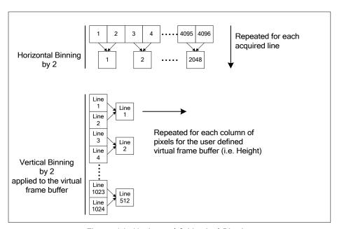
Figure 14: Horizontal & Vertical Binning
