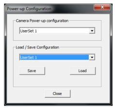
Figure 27: CamExpert - Power-up Configuration Dialog
