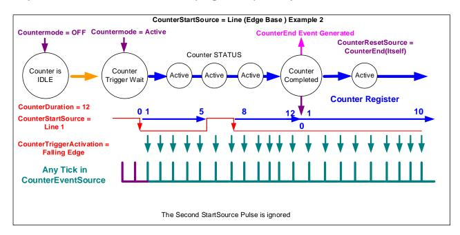
Figure 53: Example - CounterStartSource = Line (Edge Base)
