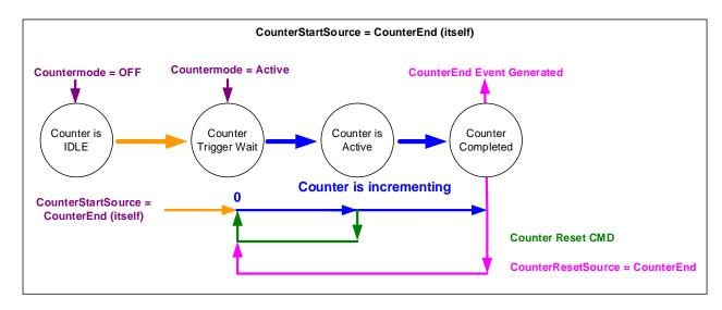
Figure 50: Example - Counter Start Source = CounterEnd
