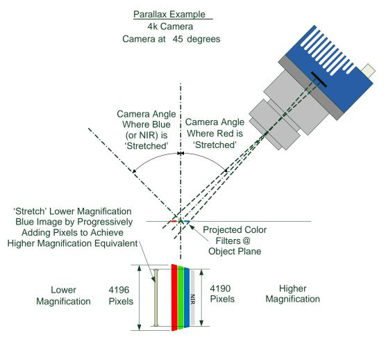
Figure 38: Camera Angle Creates Parallax
