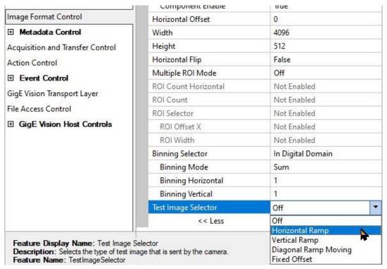
Figure 30: CamExpert - Test Image Selector
