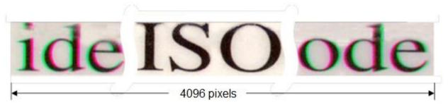
Figure 39: Image with Horizontal Color Alignment Issues
