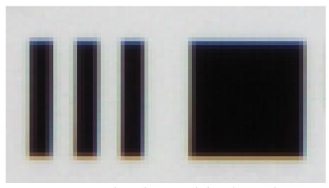
Figure 36: Color Artifacts Example (encoder 19 μm)
