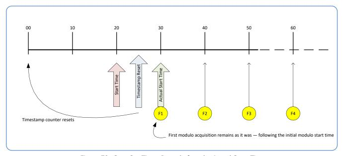
Figure 70: Case 3 - Timer Reset before the Actual Start Time
