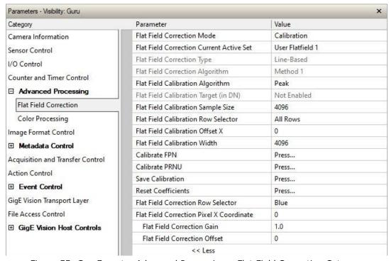
Figure 55: CamExpert - Advanced Processing - Flat Field Correction Category
