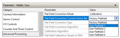
Figure 24: CamExpert - Flat Field Correction Current Active Set
