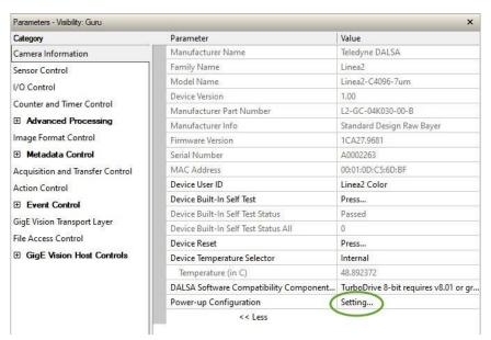
Figure 26: CamExpert - Power-up Configuration
