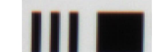
Figure 37: Color Artifacts Example (encoder 21µm)
