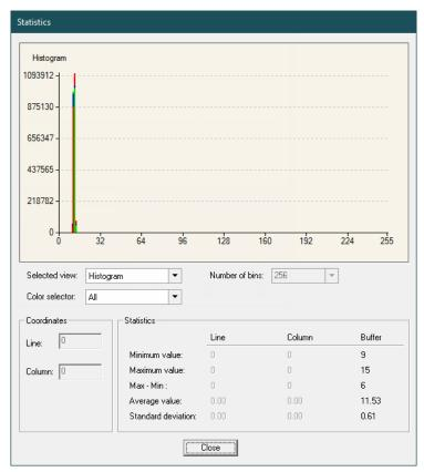
Figure 23: CamExpert Statistics Dialog - FPN Pixel Output
