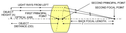
Figure 87: Primary Points in a Lens System
