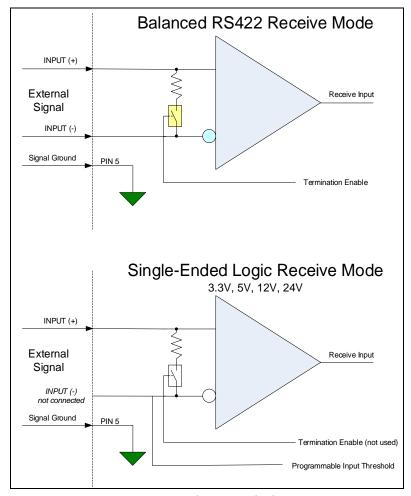
Figure 83: External Inputs Block Diagram
