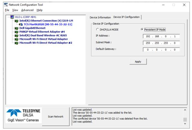
Figure 93: Network Configuration Tool - Proper IP Assigned
