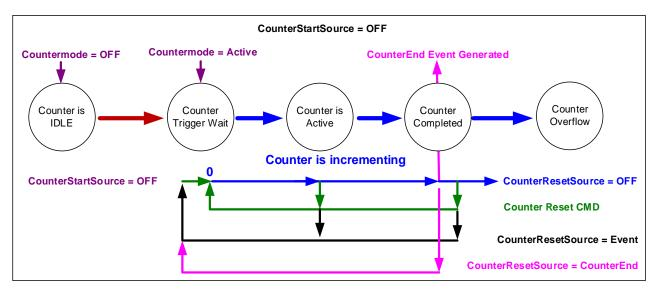
Figure 49: Example - Counter Start Source = OFF
