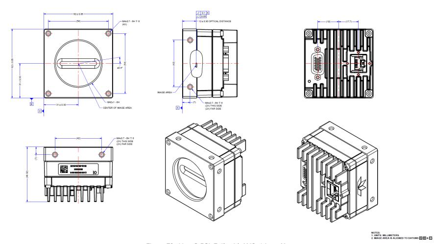
Figure 79: Linea2 5GigE 4k with M42x1 Lens Mount
