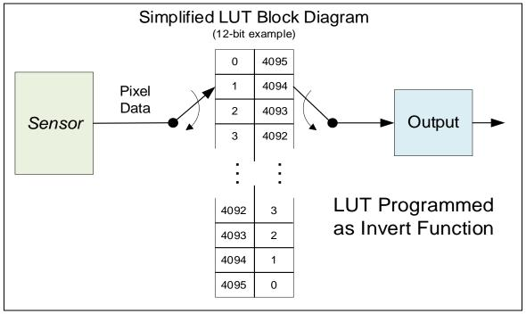
Figure 57: Example of a 12-bit LUT Invert Function
