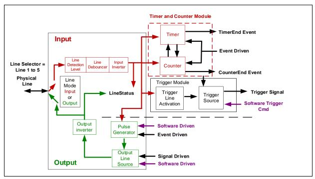
Figure 48: Counter and Timer Group Block Diagram
