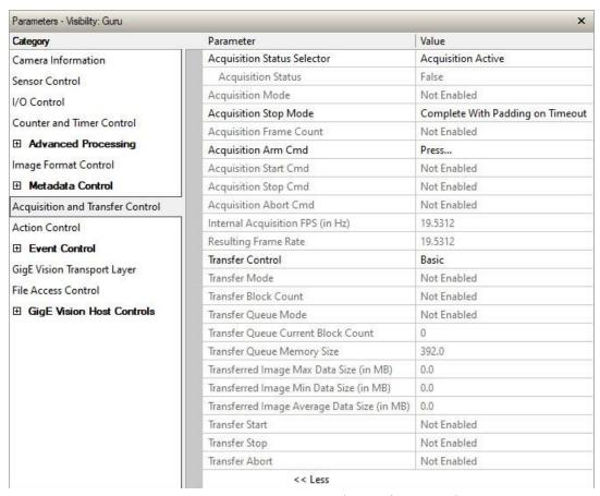
Figure 64: CamExpert - Acquisition and Transfer Control Category
