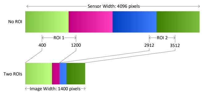
Figure 60: (Top) Test image without ROI. The entire width of the sensor is displayed. (Bottom) Multiple ROI Mode activated with two ROIs: ROI 1 has an offset of 400 pixels and is 800 pixels wide; ROI 2 has an offset of 2912 pixels and is 600 pixels wide. Both ROIs are combined to form an image 1400 pixels wide.
