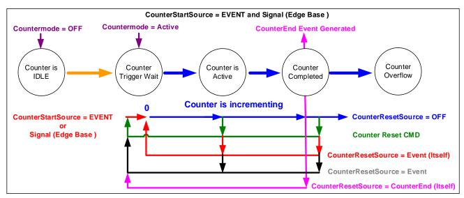
Figure 51: Example: CounterStartSource = EVENT and Signal (Edge Base)
