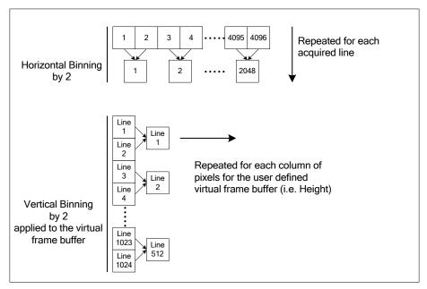
Figure 42: How Binning Works
