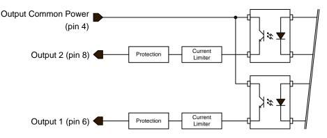
Figure 65: External Outputs Block Diagram
