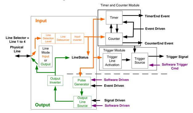
Figure 19: I/O Module Block Diagram
