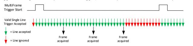
Figure 22: 10-Line Single Frame Trigger Example
