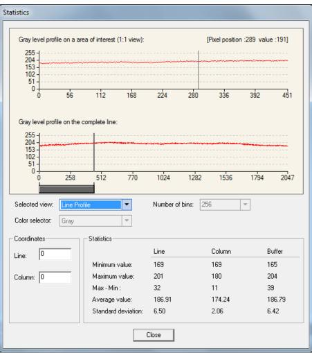
Figure 34: Bare Image Line Profile of a White Uniform Object
