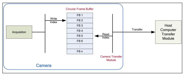
Figure 47: Camera Circular Frame Buffer
