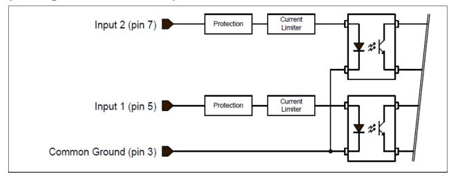
Figure 60: External Inputs Block Diagram
