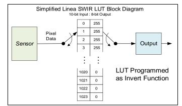
*Figure 31: Simplified Example of a 10-bit to 8-bit LUT invert function.*
