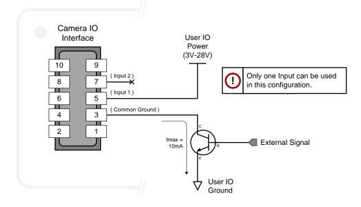
Figure 63: External Inputs with Common Emitter Sources
