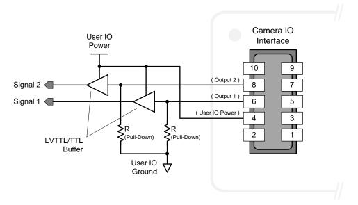
Figure 67: External Outputs with External TTL/LVTTL Drivers
