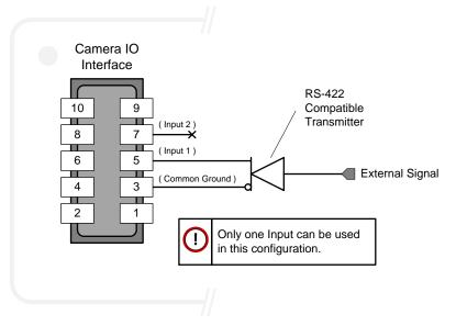
Figure 64: External Inputs with Balanced Driver Source
