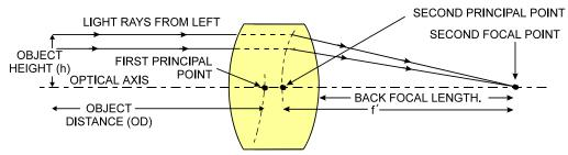
Figure 73: Lens System Diagram
