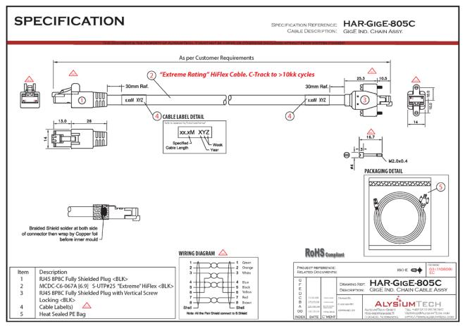
Figure 84: "Extreme Rating" HiFlex Ethernet Cable
