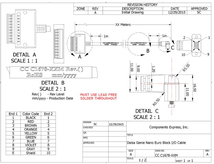
Figure 81: Cable Assembly: Right-Angle I/O to Euro Block
