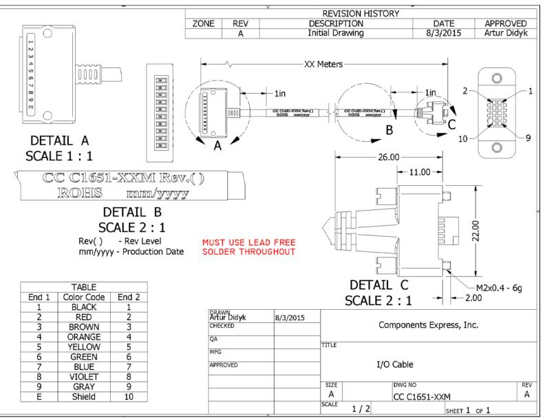
Figure 77: Cable Assembly G3-AIOC-BRKOUT2M
