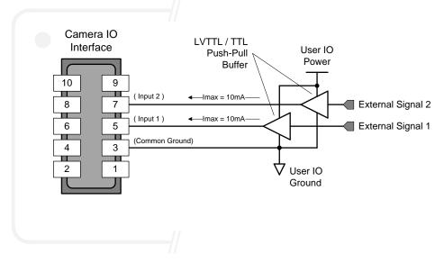
Figure 61: External Inputs with TTL Sources
