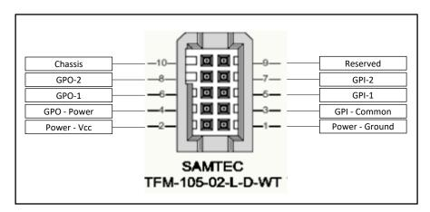
Figure 57: I/O Connector ID
