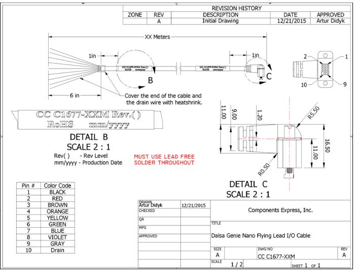
Figure 80: Cable Assembly: Right-Angle I/O Bunt End
