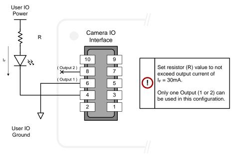
Figure 68: External Output with External Common Anode LED
