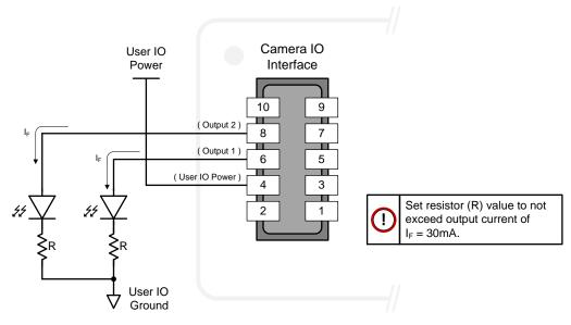
Figure 69: External Outputs with External LEDs
