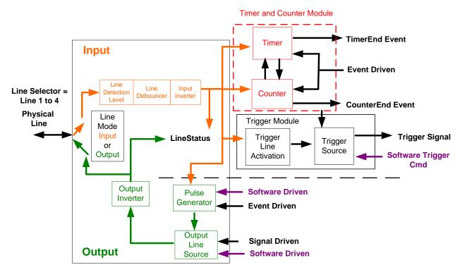
Figure 24: Counter and Timer Block Diagram
