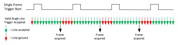
Figure 21: 10-Line Single Frame Trigger Example
