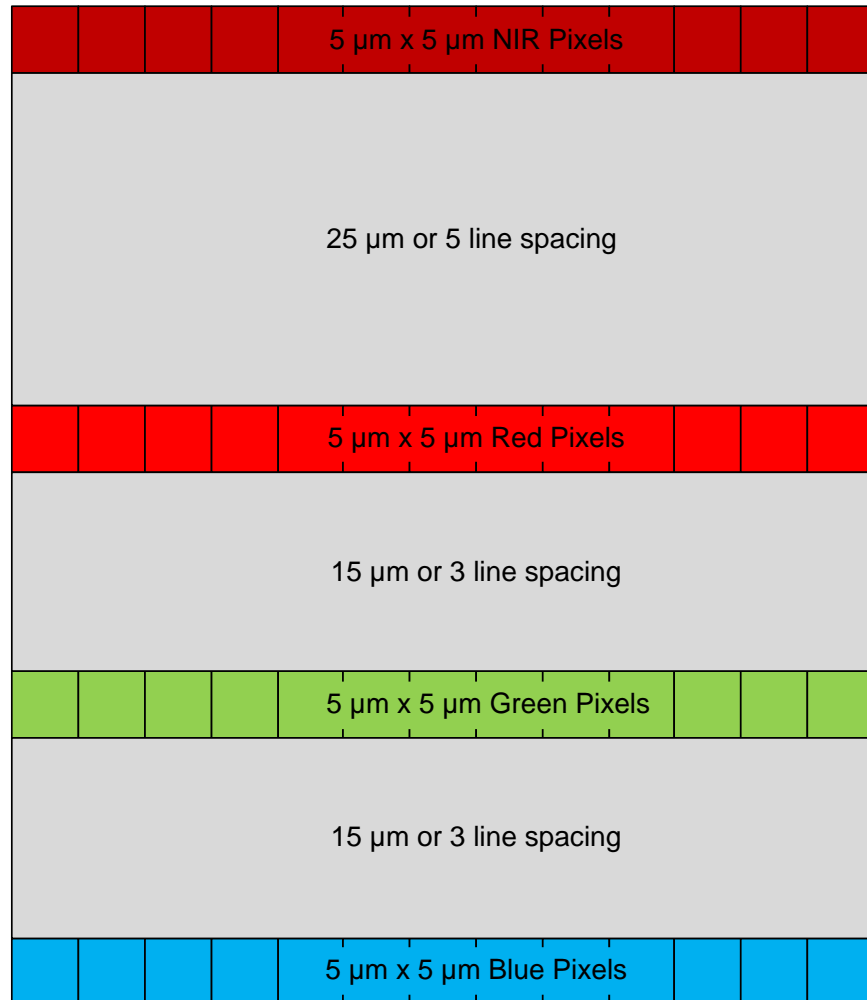
Figure 1 ML-FC-08K07N-00-R Color Pixel Structure
