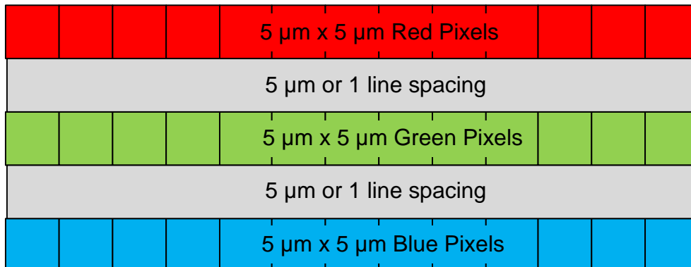
Figure 2: ML-FC-08K10T and ML-HC-16K10T Color Pixel Structure
