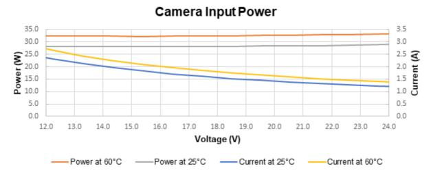
Figure 13: Super Resolution Model Power Vs. Input Voltage
