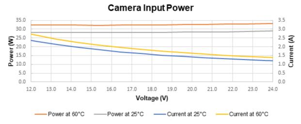
Figure 6: HL-HM-16K40H-00 Power Vs. Input Voltage
