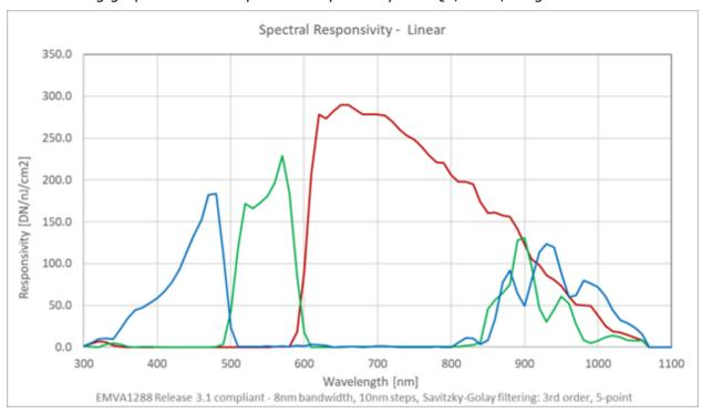
Figure 9: Multifield Model Spectral Responsivity
