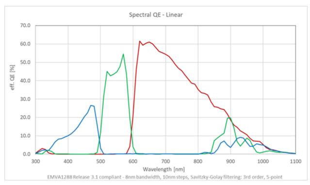
Figure 10: Multifield Model QE
