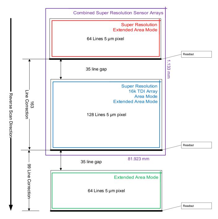
Figure 35: Super Resolution Camera Line Spacing - Reverse Scan Direction
