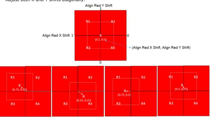
Figure 47: Align Red X Shift and Align Red Y Shift
