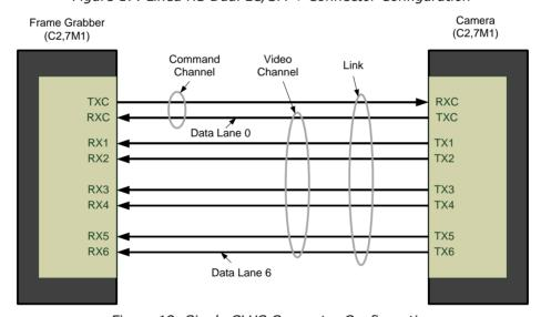
Figure 18: Single CLHS Connector Configuration
