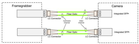
Figure 17: Linea HS Dual LC/SFP+ Connector Configuration
