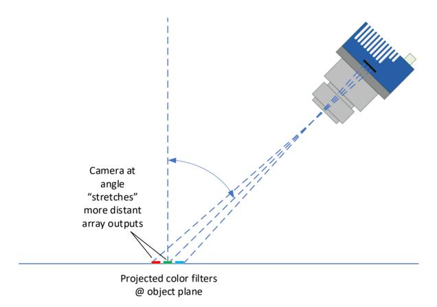
Figure 37: Camera Angle Parallax
