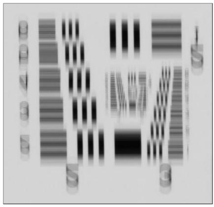
Figure 27: Image with incorrect scan direction
