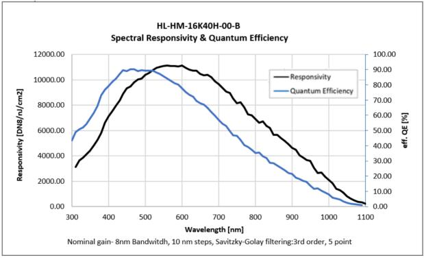
Figure 3: 16K Monochrome Models Spectral Responsivity & QE
