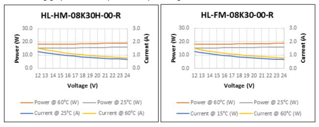
Figure 4: Standard 8K Models (CX4 and SFP+) Power vs. Input Voltage
