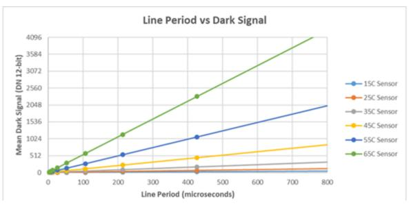
Figure 15: Line Period vs. Dark Signal
