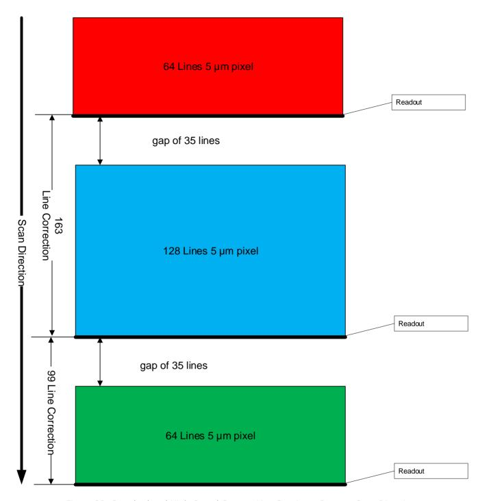
Figure 33: Standard and High-Speed Camera Line Spacing – Reverse Scan Direction
