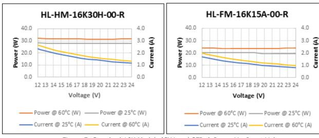
Figure 5: Standard 16K Models (CX4 and SFP+) Power Vs. Input Voltage
