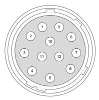
Figure 25: 12-pin Hirose Pin Numbering
