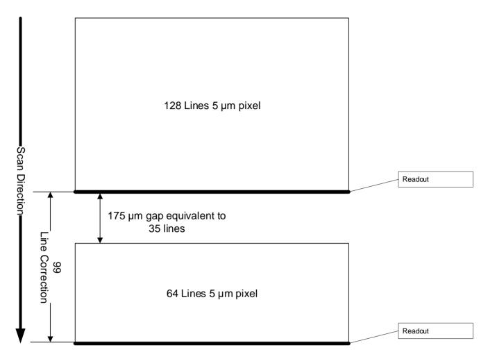
Figure 31: Standard and High-Speed Camera Line Spacing – Reverse Scan Direction
