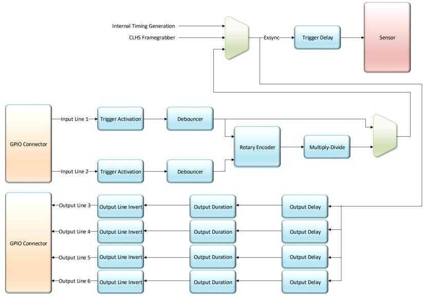
Figure 40: GPIO functionality block diagram
