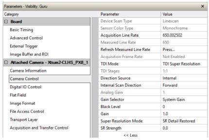
Figure 52: Camera Control Panel
