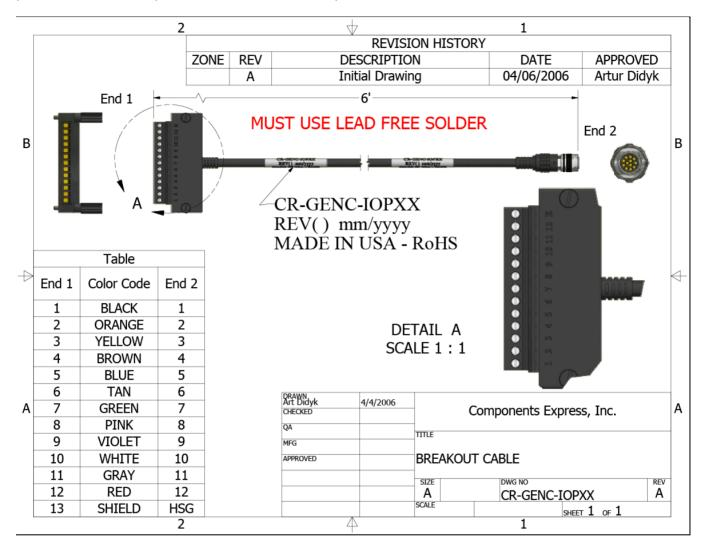
Figure 26: GPIO cable accessory #CR-GENC-IOP00
