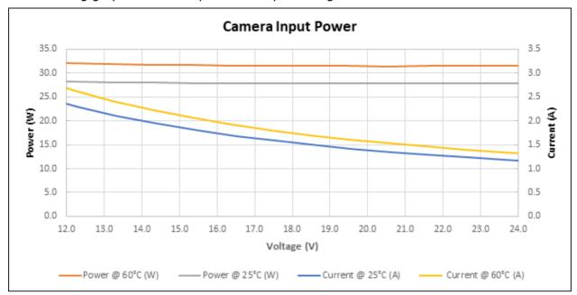
Figure 8: Color Model Power Vs. Input Voltage
