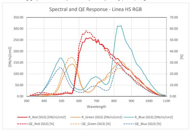
Figure 7: Color Model Spectral Responsivity and QE
