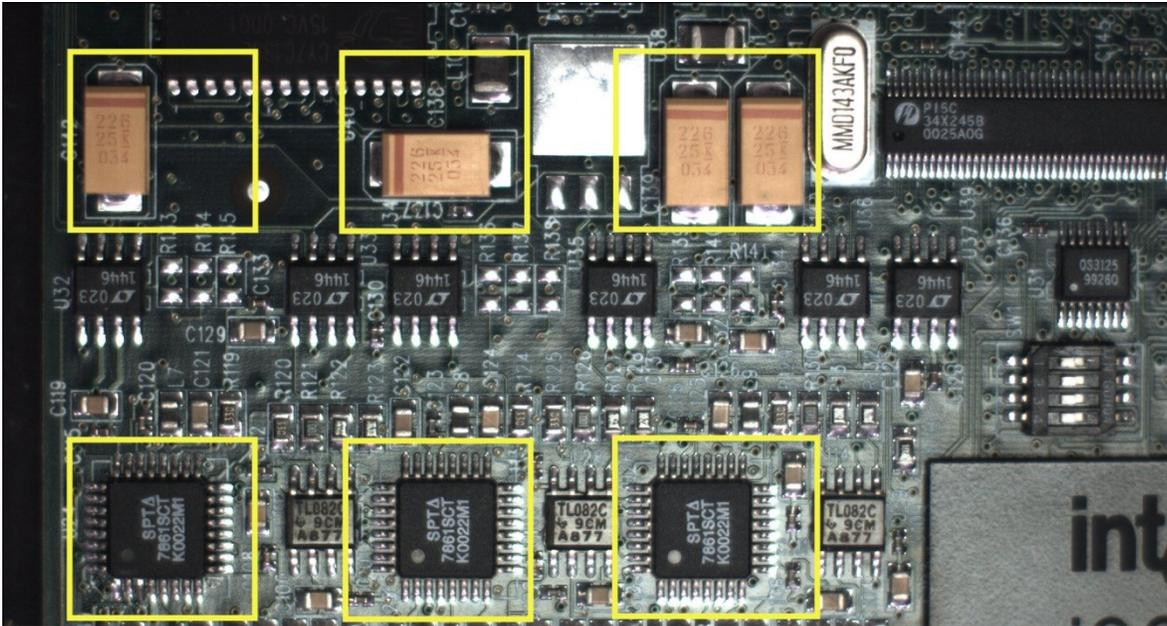
With the ROI areas defined, the camera outputs an image consisting only of data within those ROI areas, as shown below. Such data reduction improves transfer bandwidth and also reduces image processing time for the host system imaging application.
