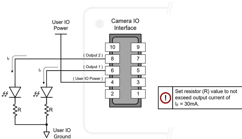
⚠ Set resistor (R) value to not exceed output current of  $I_F = 30\text{mA}$ .
