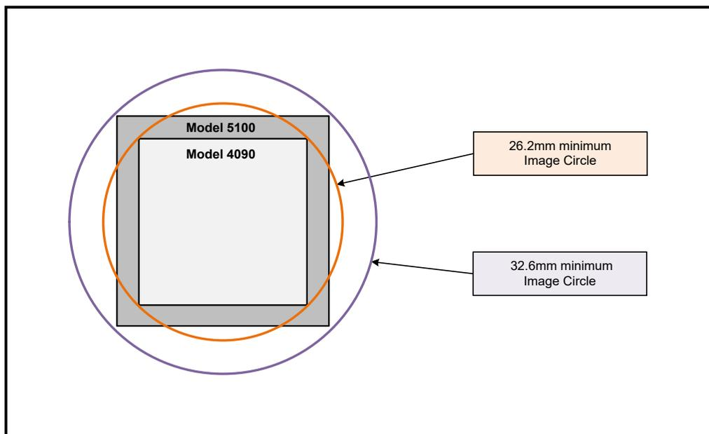
The following figure shows the lens image circles relative to Genie Nano-CXP models using the Teledyne E2V Emerald 37.7M (Four Thirds image sensor format) and 67.1M (APS-C image sensor format) sensors.
