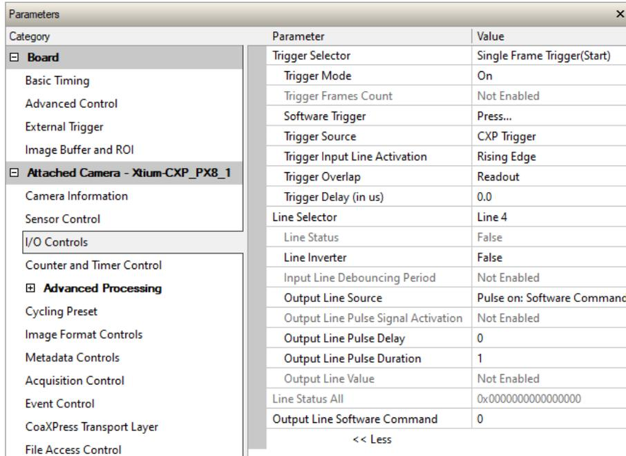
The screenshot shows the 'Parameters' dialog box with the 'Attached Camera - Xtium-CXP\_PX8\_1' category selected. The 'I/O Controls' sub-category is expanded, showing a list of parameters and their values.
