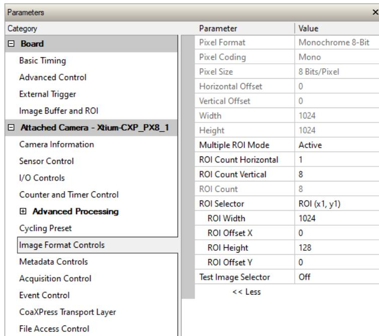
The screenshot shows a 'Parameters' dialog box with a tree view on the left and a table on the right. The tree view is expanded to 'Image Format Controls' under the 'Attached Camera - Xtium-CXP\_PX8\_1' category. The table on the right lists various parameters and their values.
