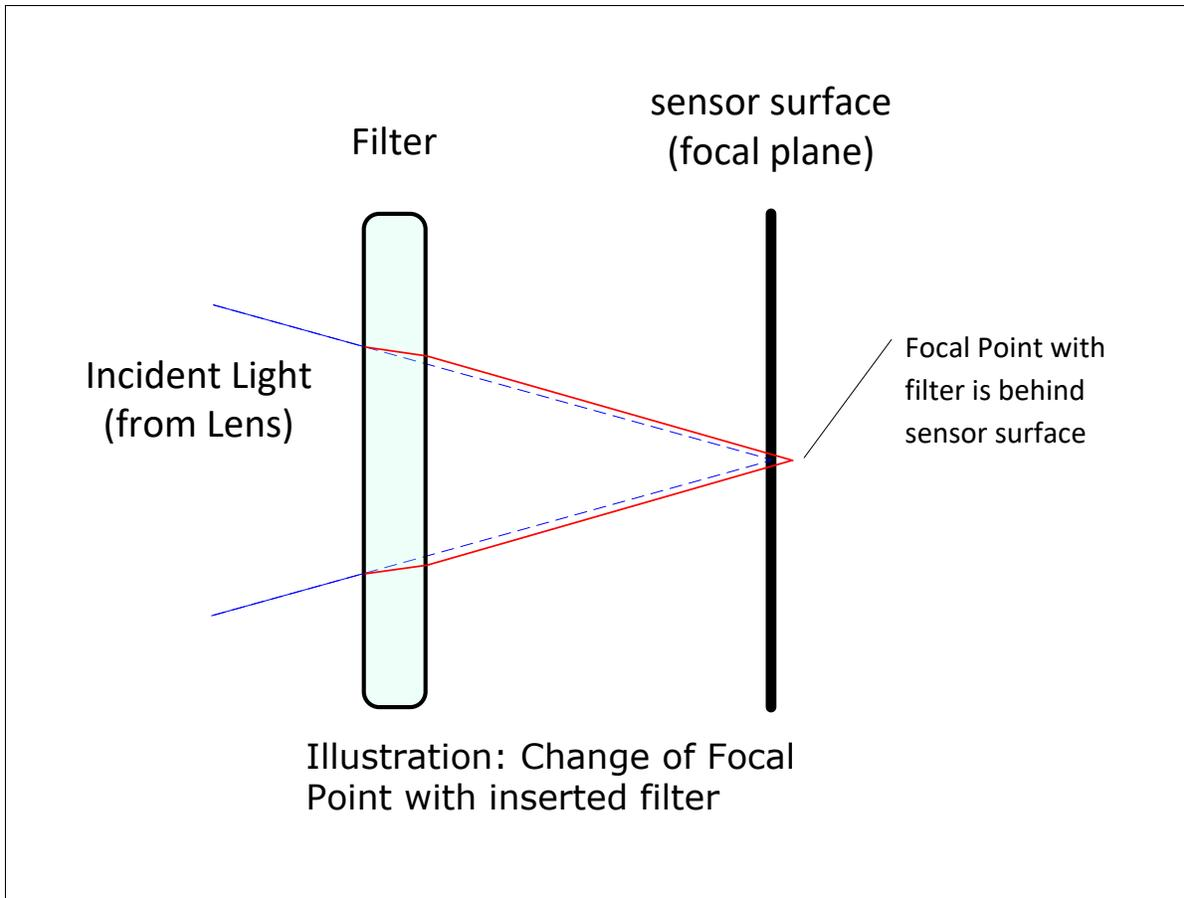
In this example when a glass filter is inserted between the lens and the camera sensor, the focal point is now about 1/3 of the filter thickness behind the sensor plane. Genie Nano filters are specified as 1mm thick.
