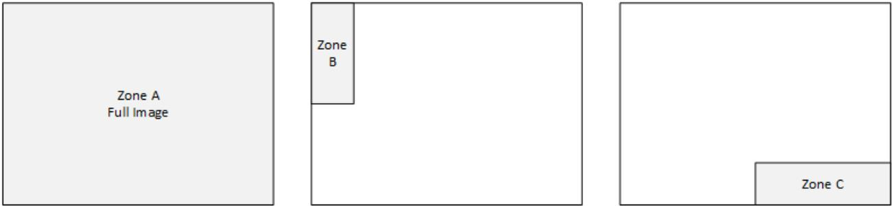
Thresholds for each of these zones can be specified; when performing an FPN correction if the values exceed any of these thresholds, the Calibir assumes an internal shutter error has occurred and attempts to close the shutter again.
