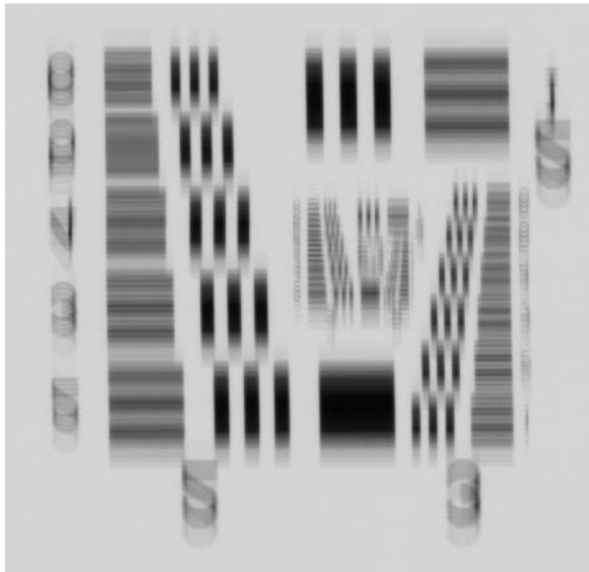
Figure 12. Image with incorrect scan direction
