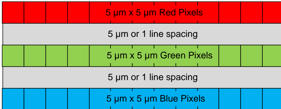
Figure 2: Linea ML Color Pixel Structure
