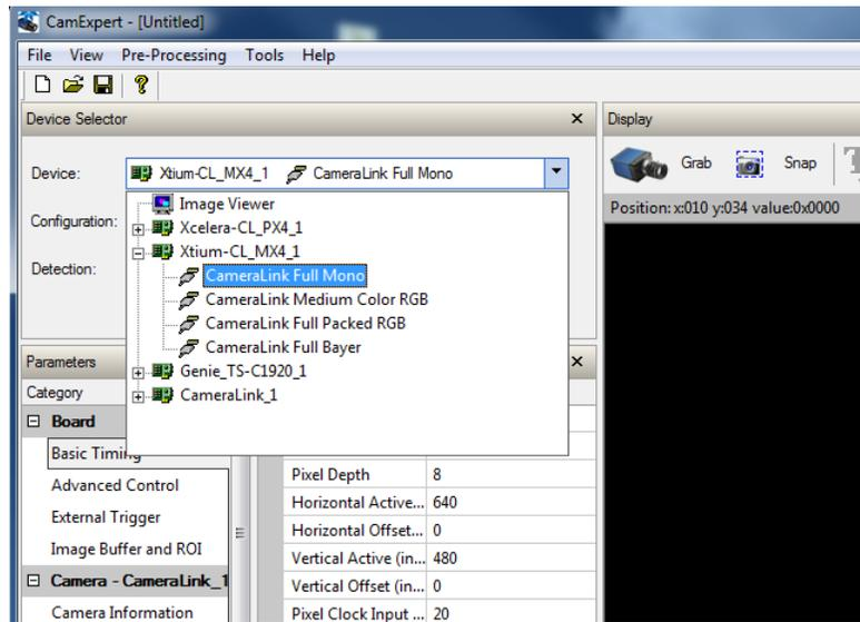
8. Modify the camera and frame grabber parameter settings as required. At present, when using GenCP cameras, the camera and frame grabber parameters must be adjusted separately. Test the image acquisition by clicking the **Grab** button.
