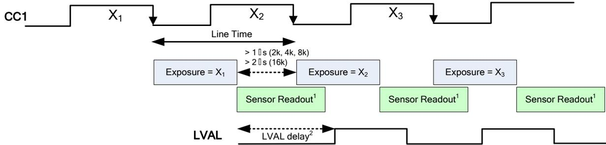
1. Sensor readout time = 12.5μs (2k, 4k, 8k) or 20.8μs (16k)
