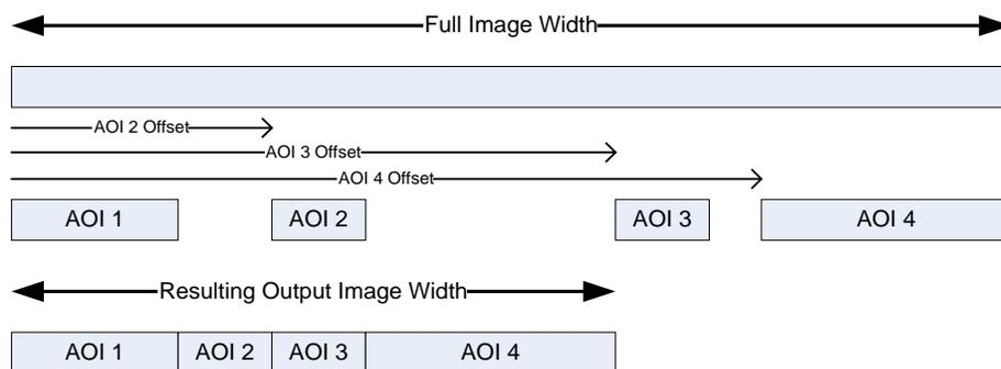
For example, in the 4k camera model, if the total number of pixels for the specified AOI's is less than 1 K when using base Camera Link mode at 77 MHz, the maximum line rate can be 80 kHz; versus 56 kHz if all 4k pixels were output.
