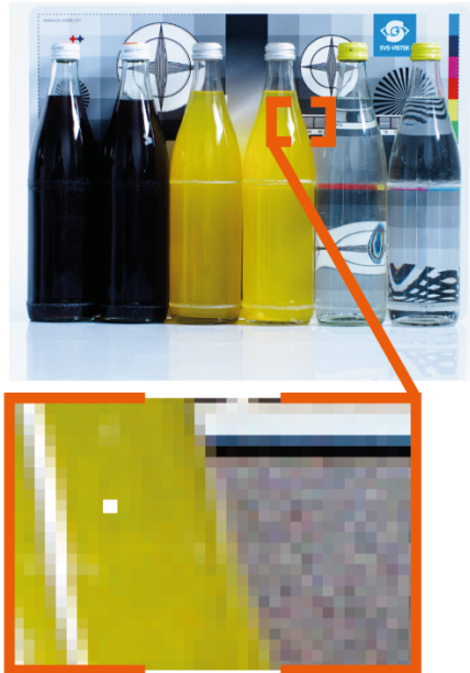
Fig. 5-20: Illustration of a defect pixel
