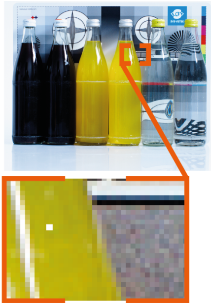
Fig. 5-23: Illustration of a defect pixel
